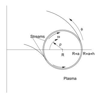
Stream function *i* of electric current in the stream
