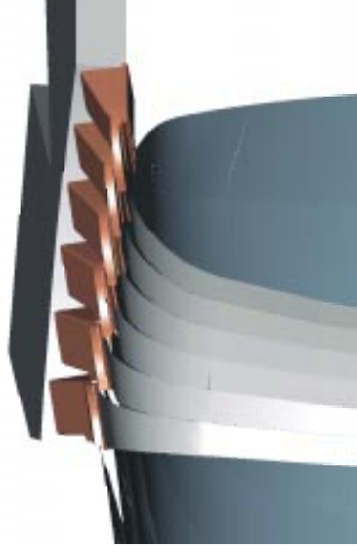
View from centerline of machine showing inclination of nozzles
