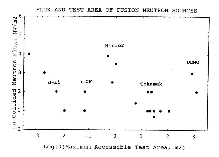
Figure 2. Maximum accessible test area and the un-collided neutron loading averaged over the test area for the VNS concepts presented at the workshop ("•" representing values from Tables 2 and 3). The values for a DEMO, and the high-flux neutron sources based on d-Li target and µCF are included for contrast.
