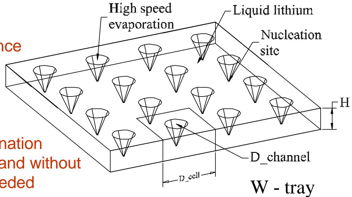
Schematic of vapor channels (side view)
