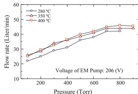
**Fig. 5.** Flow rate of PbLi as a function of temperature and argon-gas pressure.
