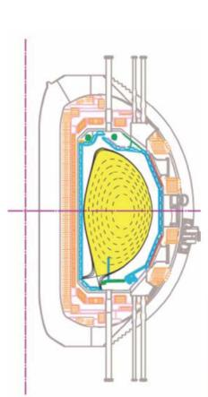
High elongation, high triangularity double null plasma shape for high gain, steady-state plasma operation
