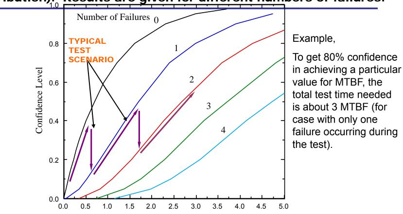
Test Time in Multiplies of Mean-Time-Between-Failure (MTBF)
