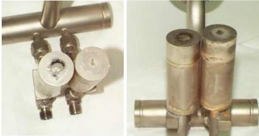
Fig. 9. Post-test photos of modules showing reflow of misplaced braze material on surface.
