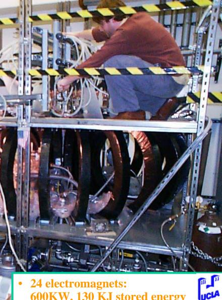
24 electromagnets: 600KW, 130 KJ stored energy
