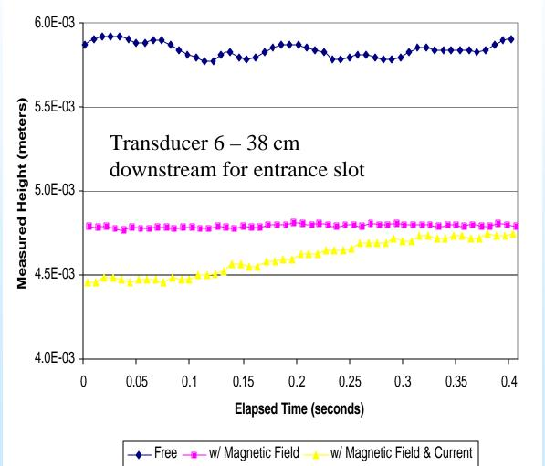
B field acts to laminarize flow – **Reducing flow resistance and eliminating surface waves**
