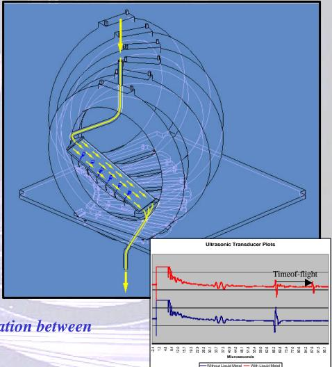
Example results from MTOR Experiments: Film flow height response to toroidal field and magnetic propulsion current
