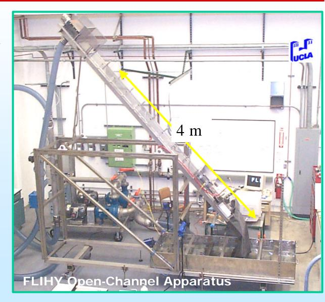
**Example of FLIHY EXPERIMENTAL RESULTS: SURFACE WAVINESS is the KEY FACTOR for HEAT TRANSFER in Free-Surface Turbulent Flows**
