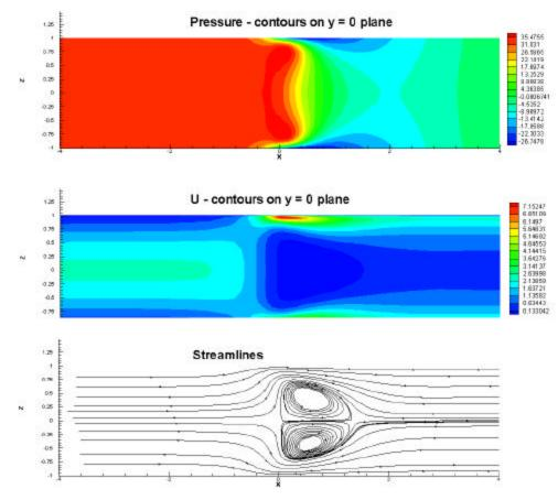
Channel flow in a fringing magnetic field: Ha=1000. 3-D calculations by HIMAG code. Two trapped vortices can be seen.
