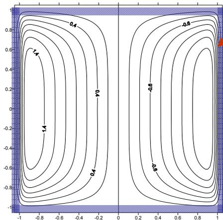
Lines of current enter the low resistance wall – leads to very high induced current and high pressure drop
