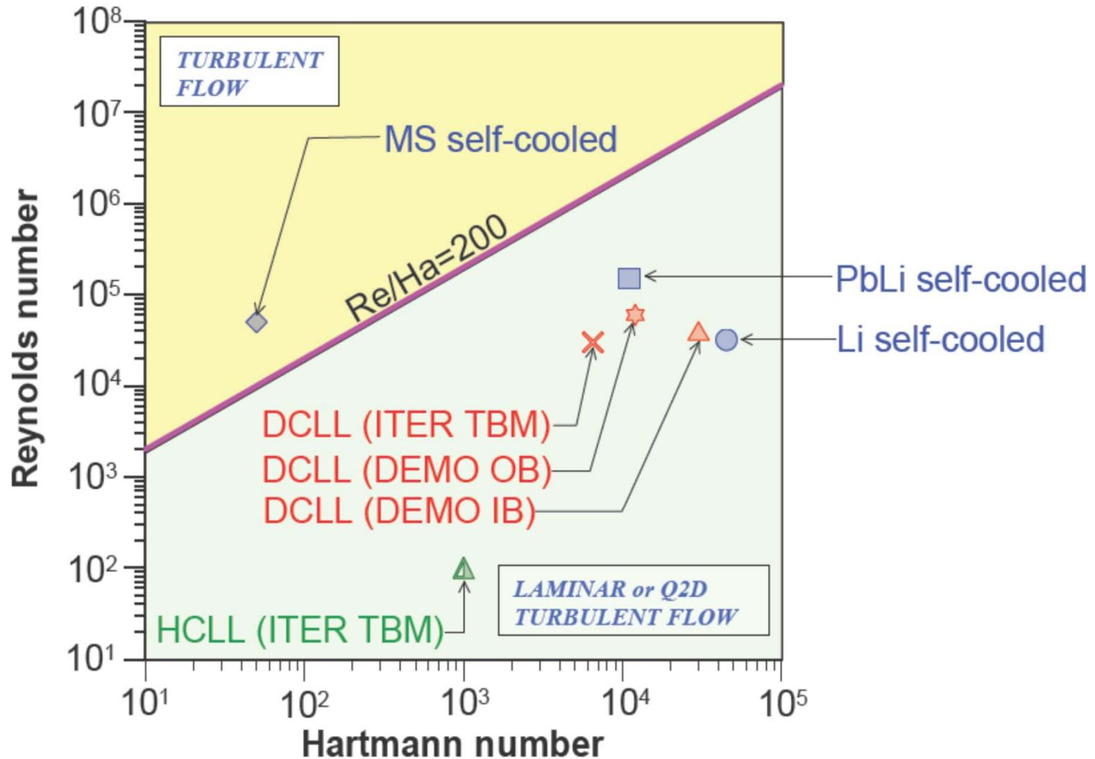
**Self-Cooled liquid metal blankets are NOT feasible now because of MHD Pressure Drop**
