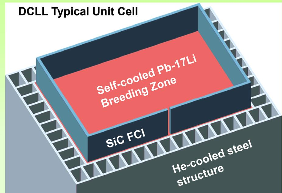
***Pb-17Li exit temperature can be significantly higher than the operating temperature of the steel structure ⇒ High Efficiency***
