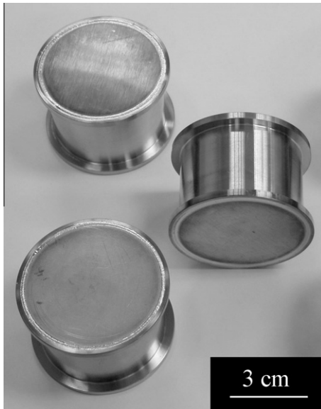
Fig. 1. HIP cans after closure, prior to HIP cycle.
