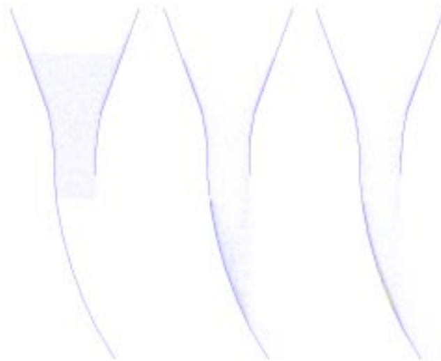
Figure 9.3.4-1. Flow from a high-porosity inlet condition
