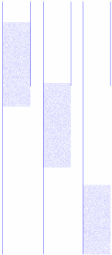
Figure 9.3.3-1. Flow geometry in a vertical chute with uniform initial condition
