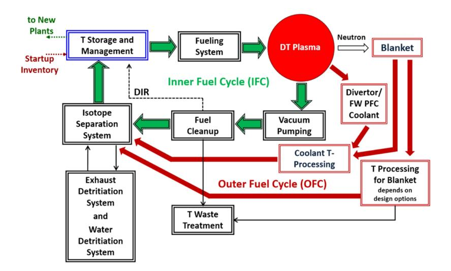
Simplified Schematic of the D-T Fuel Cycle
