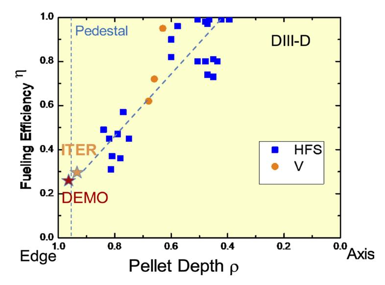
Fueling Efficiency Extrapolation from Deep to Shallow Penetrating Pellets Expected in ITER and DEMO is Highly Uncertain. Extrapolation shows fueling efficiency  $\eta < 25\%$  in ITER and even lower in DEMO Serious Consequences for required T start up and self-sufficiency
