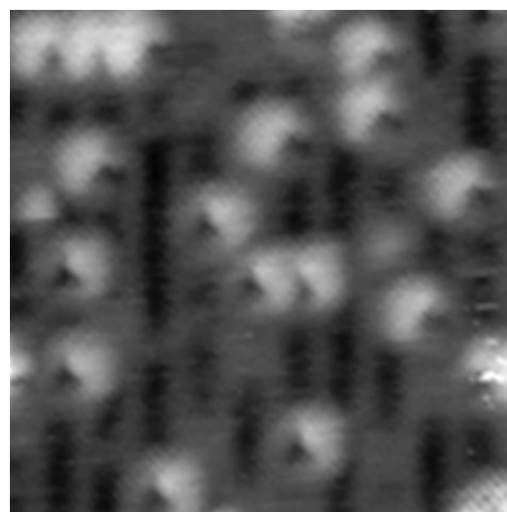
Figure 3. High-resolution STM image ( 70 \times 70 \text{Å}^2 ) exhibiting strong trigonal intensity contrast within each (\text{WO}_3)_3 cluster. One of the corners aligns with a \text{Ti}^{\text{IV}} row and the opposite side is tilted with equal probability to the left or right away from this row.
