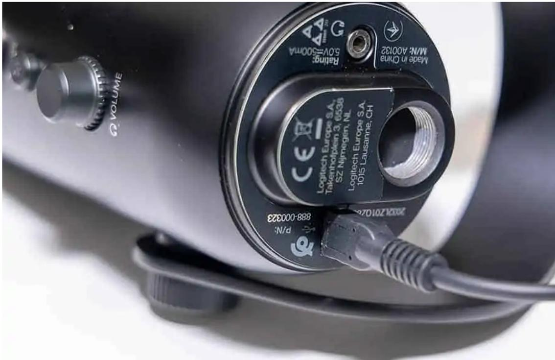
USB cable connected to the mini USB socket on the base of the Blue Yeti
