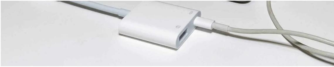
Pass-through power supplied by connecting a power bank to the camera adapter
