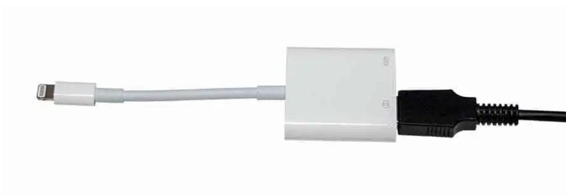
Blue Yeti USB cable connected to Apple Lightning to USB 3 Camera adapter
