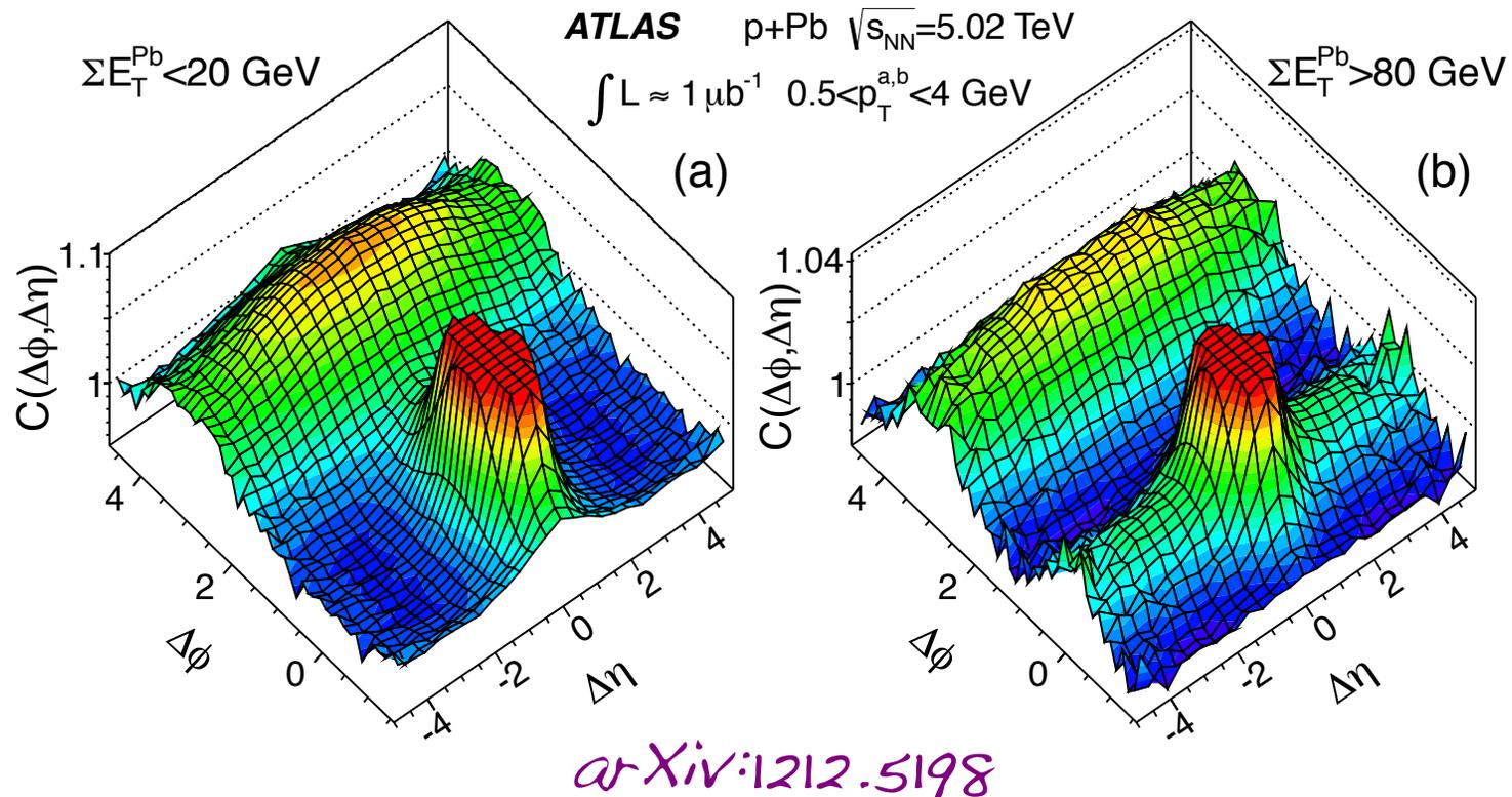
Central collisions (right) also show a **ridge** near  $\Delta\Phi=0$ , similar to that observed in Pb-Pb collisions. Fluid?
