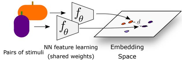
Figure 1: DrLIM is a twin (or “Siamese”) deep metric learning network that uses two identical networks  $f$  with shared parameters  $\theta$  to project pairs of stimuli into an embedding space. The network is then trained to minimize the error of predicting same-different judgments for all pairs, given the distance  $d$  in the embedding space.
