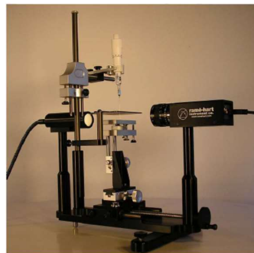
Interfacial Tension by Pendant Drop
