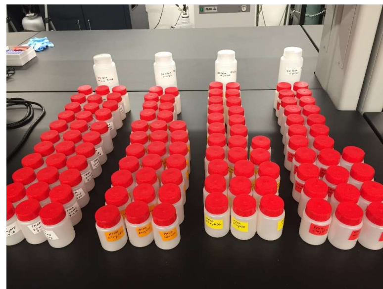
PFOA and PFOS working solutions from 0.1 to 10,000 mg/L in 100-mL HDPE bottles
