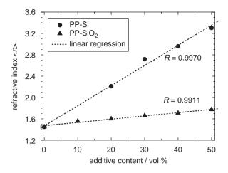
Fig. 3. Refractive index  $\langle n \rangle$ , averaged in a dependable frequency range, over volumetric content of the additives silicon and silica in polypropylene: a linear correlation can be assumed.
