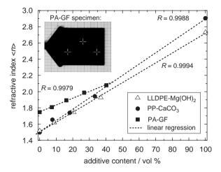
Fig. 2. Refractive index  $\langle n \rangle$ , averaged in a dependable frequency range, over volumetric content of the additives magnesium hydroxide, calcium carbonate and glass-fibres in standard polymers: the regressions and their correlation coefficients R lead to the assumption of a linear dependency.
