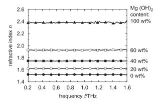
Fig. 1. Refractive index over frequency in the terahertz range with different magnesium hydroxide content (wt%) in LLDPE.
