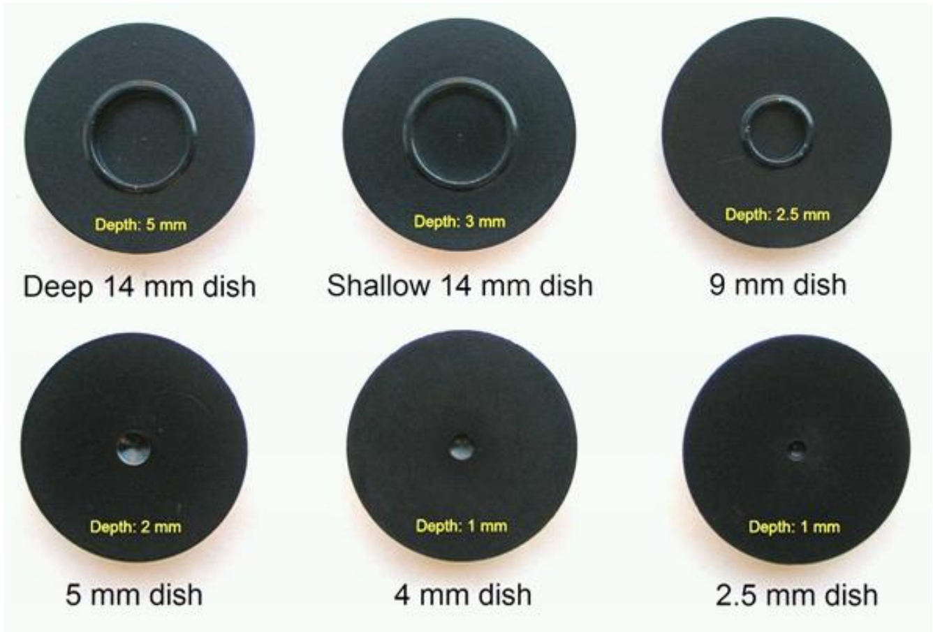
Fig. 1. Black dishes for particular samples mounted on the multiple-spinning stage shown in Fig. 2.
