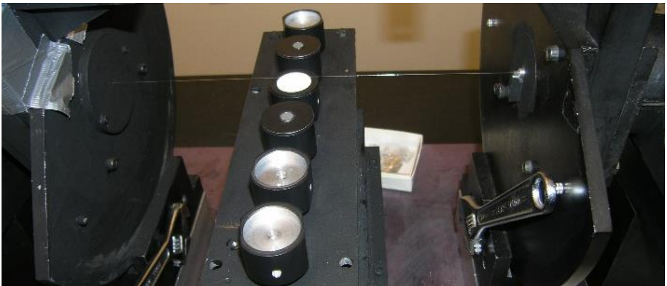
Fig. 2. Multiple-spinning stage that allows up to five samples measured along with the standard material (Spectralon) while being spun at a rate of 1.5 seconds per rotation.
