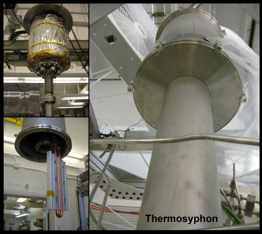
Thermosyphon nitrogen Closed loop condensation/evaporation. Provides 1 kW cooling power to the detector.
