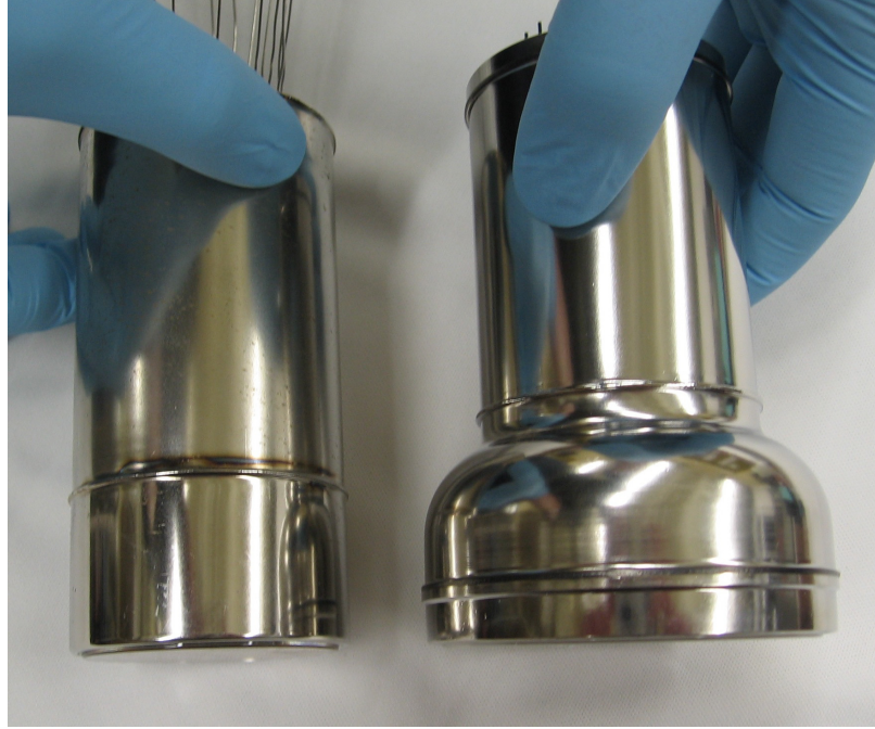
Figure 7.9: The Hamamatsu R8778 PMT, used in LUX (left), and the R11410-20 PMT, used in the upcoming LZ experiment (right). The R11410-20 features a 6.4 cm diameter photocathode, offering twice the surface area of the 4.5 cm diameter R8778 photocathode.
