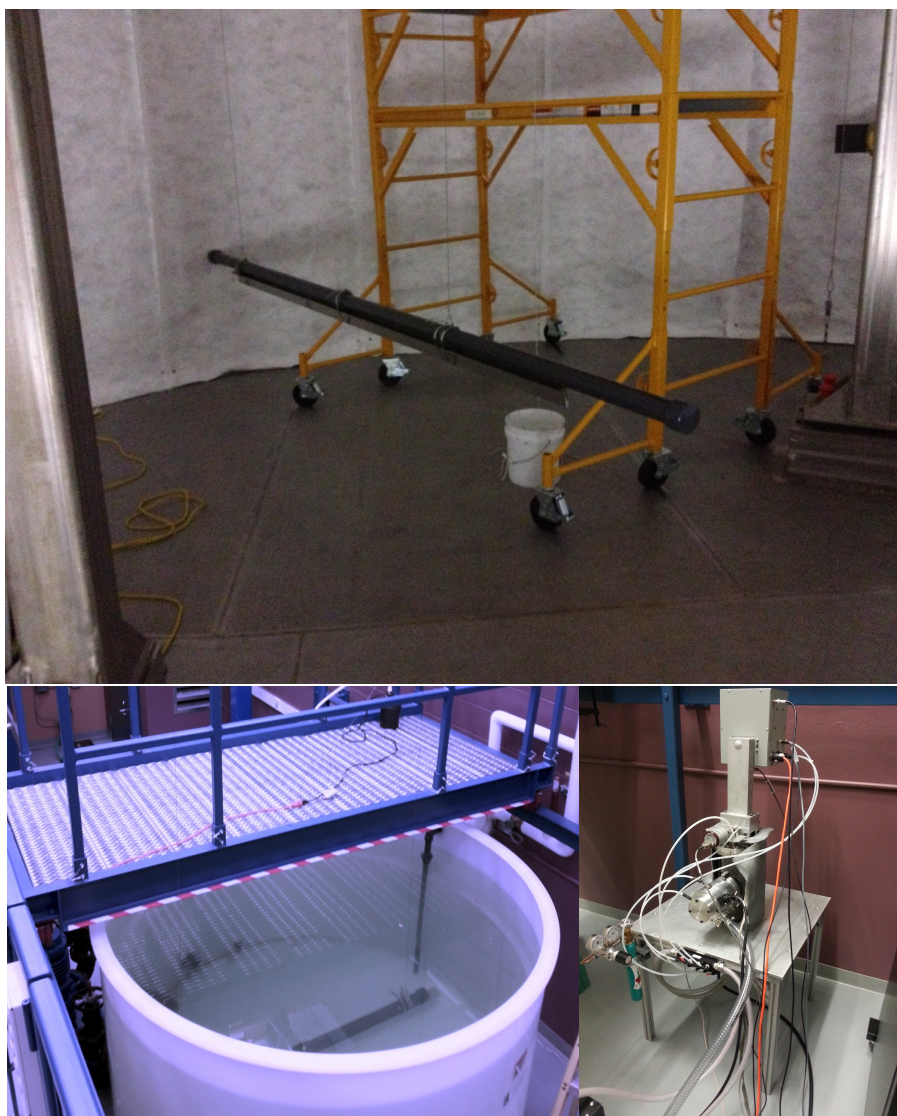
Figure 4.2: (Top) The fully assembled neutron conduit in the LUX water tank. The PVC body measures 377 cm end-to-end, with 4.9 cm inner diameter. A stainless steel T-bar is used for ballast. Stainless steel hose clamps secure the pipe to the ballast in three locations to prevent bowing. Stainless steel wire connects the tube to winches at the top of the water tank, allowing operators to raise and lower the conduit during calibration operations. (Bottom Left) The 1 m prototype tube, used to test sealing, ballast and suspension techniques. The tube is immersed in the 1.8 m height water tank at Brown University. (Bottom Right) The DD-108M neutron generator, during initial testing at Brown. The generator head is located in the middle of the tee, in line with the turbopump.
