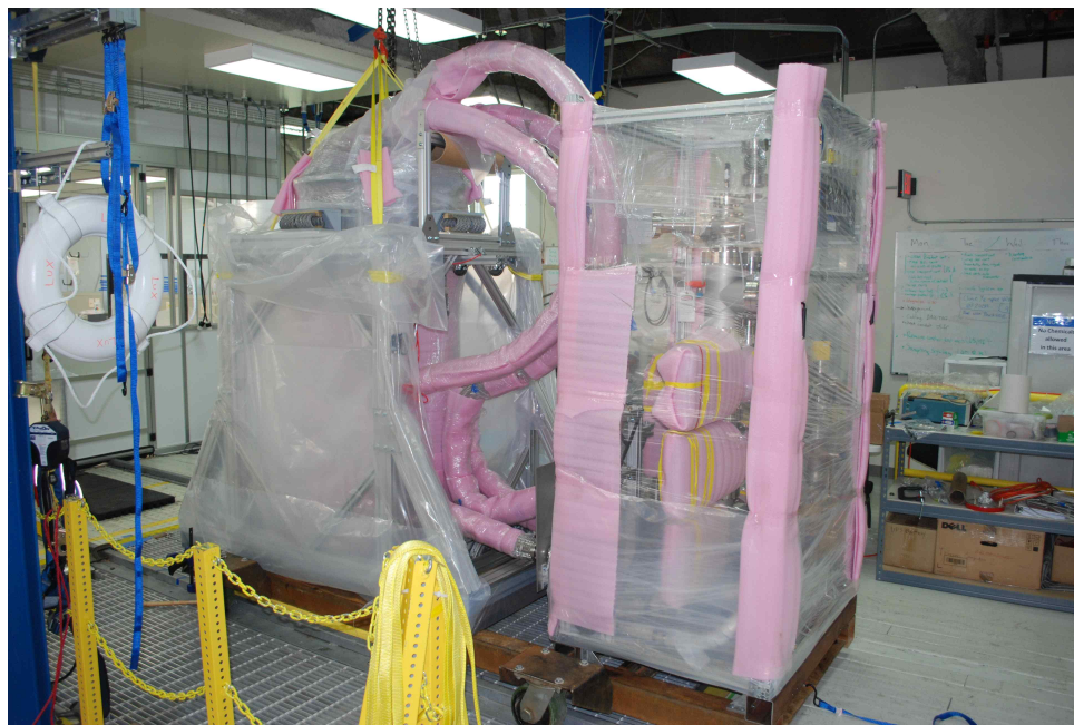
Figure 2.8. The LUX detector is packaged and ready to leave the surface facility. On the left is the detector on its transport cart, and on the right is the instrumentation breakout. The three umbilicals are visible. Everything is packaged in plastic and foam to keep dust off. Photograph by Jeremy Mock.
