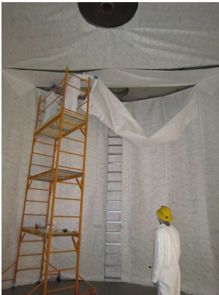
Figure 2.4. The interior of the LUX water shield. Tyvek panels are being applied to the sides and top of the tank as this material is highly reflective of the Cherenkov photons that are produced when a high energy muon enters the water. 20 ten inch photomultiplier tubes complete the veto system.
