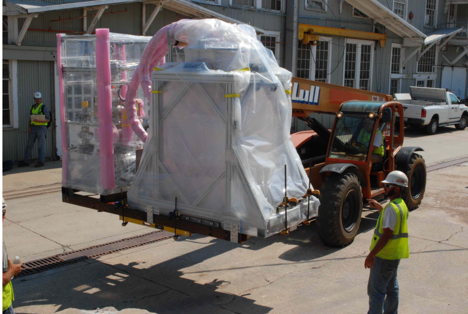
Figure 2.9. The LUX detector and instrumentation system, attached as a unit, are being transported from the surface assembly facility to the building where they will be loaded into an elevator to go underground. During this 1000 foot trip, the unit never experienced any external forces (except gravity) and was never tilted more than one degree from the horizontal. Photograph by Matt Kapust.
