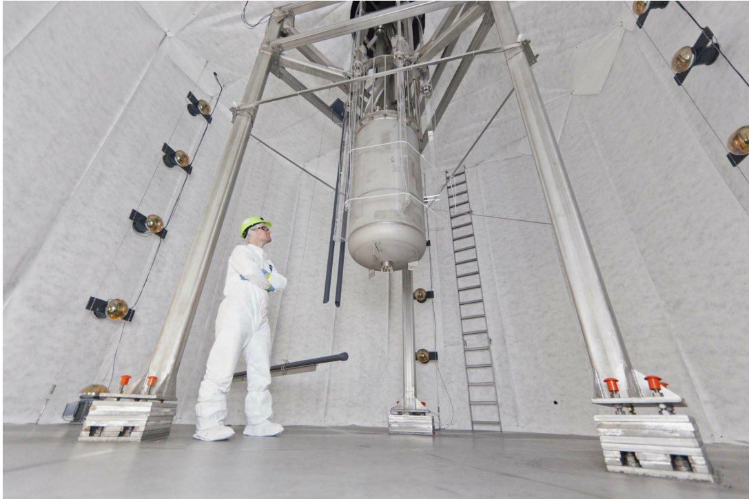
Figure 2.12. The LUX detector installed in the water shield. The weight is fully supported by the detector stand, the large structure mounted to the floor of the tank. The detector hangs from the support ring. Above the support ring is the infrastructure that delivers cryogenics and circulation systems. The tube in the background guides calibration neutrons into the active volume (discussed in later chapter). The scientist in the photo is the author, Jeremy Mock. Photograph by Matt Kapust.
