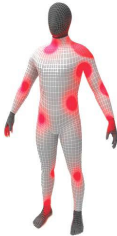
Fig. 3: EMU injury hotspots. Conceptual representation of the areas where injuries and pressure contact points most often occur.
