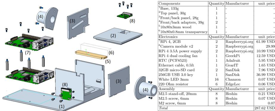
Fig. 2: Left: Exploded view of the entrance; numbers relate to superscripts in the table on the right. The cameras are mounted  $\sim 55$ mm from the tunnel surface. Note that all components are also available on Amazon, except for the 3D printed pieces produced with PLA at 21.99 USD/kg. For assembly, users need a screwdriver, a box cutter, a needle nose plier, a soldering iron, a screen, and the ability to program the micro-SD cards.
