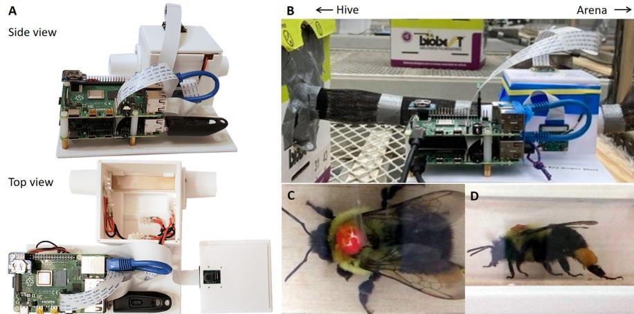
Fig. 1: Automated entrance monitor (A-B) capturing top and side photos (C-D) of bumble bees as they enter and exit their hive; the bee shown is carrying pollen. Note that to fit this article, all photos have been post-cropped.
