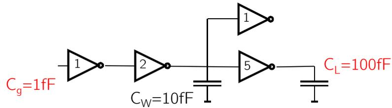
$$t_{p,i} = t_{p0} \left( 1 + \frac{C_{ext,i+1}}{\gamma C_{g,i}} \right) \quad \gamma = 1 \quad t_{p0} = 3ps$$
