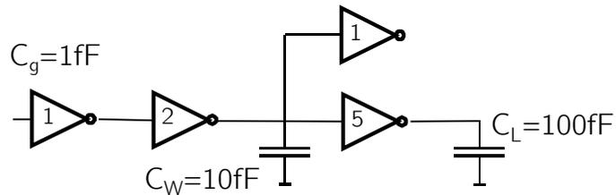
$$t_{p2} = t_{p0} \left( 1 + \frac{C_g + 5C_g + 10fF}{2C_g} \right) = t_{p0}9$$
