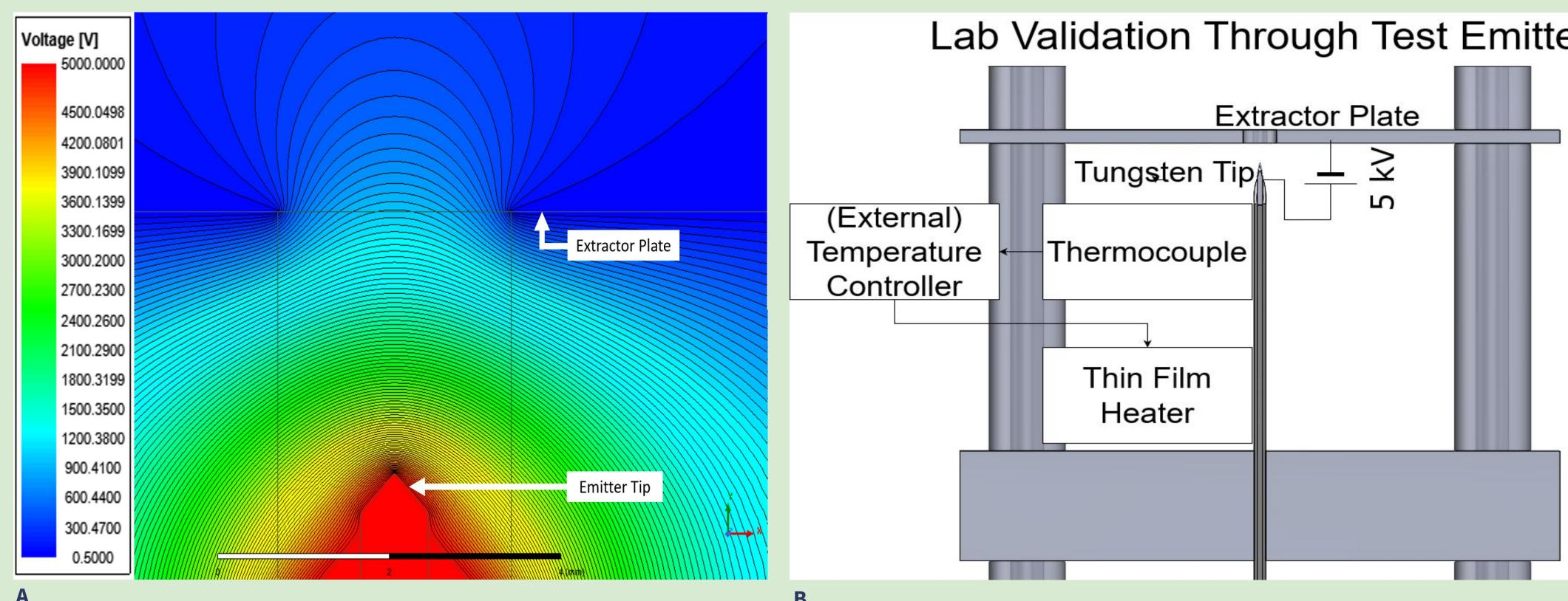
(A) Voltage contours produced around an operating FEEP tip. This map highlights the instability produced by the localized tip of the Taylor cone and the decrease in potential with increased distance from the tip (B) Cross section of CAD model, indicating the **temperature control loop** setup and power connections
