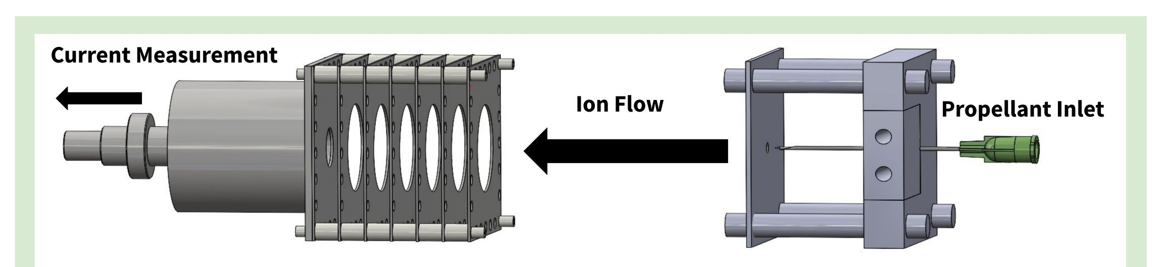
**Retarding Potential Analyzer (RPA)** The FEEP plume can be quantitatively analyzed with a retarding potential analyzer (left). The RPA can provide an **energy spectrum** of the plume being emitted from the thruster, giving us an indication of the **efficiency** of the thruster as well as quantifying **directional losse**s which may be encountered as a result of deflection of the ion plume
