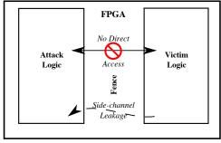
(a) FPGA-to-FPGA attacks on a shared FPGA.
