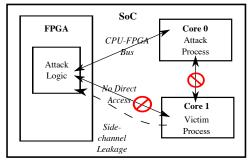
(b) FPGA-to-CPU attacks on a heterogeneous SoC.
