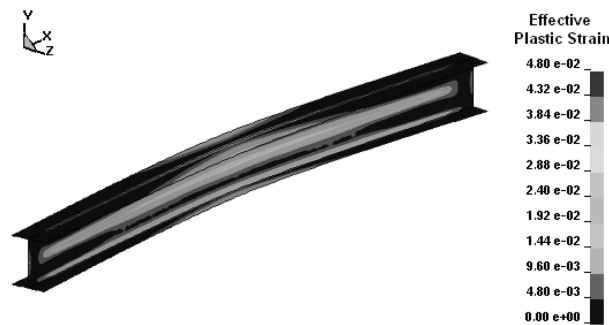
Fig. 12 Contours of accumulated effective plastic strain at t = 1 s
