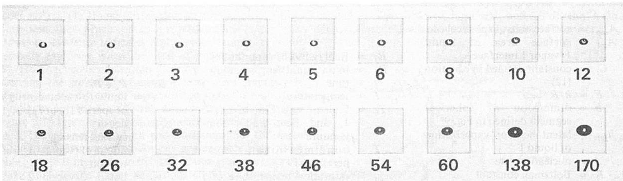
Fig. 4 N-octane droplet boiling in glycerine at  $P_0 = 1.22$  MPa. Number of frame in the motion picture sequence is shown below each photograph.  $T_0 = 531^\circ\text{K}$ ,  $R_0 = .3$  mm, framing rate = 900 frames/s.
