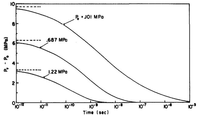
Fig. 10 Calculated variation of  $\Delta P$  with time at pressures  $P_0$  of .101 MPa, .687 MPa, and 1.22 MPa for an n-octane droplet ( $R_0 = .3$ mm). Small and large time asymptotes correspond to the nucleation pressure and saturation pressure ( $P_v = P_0$ ), respectively.
