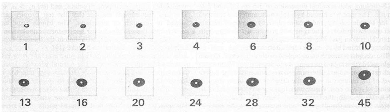
Fig. 3 N-octane droplet boiling in glycerine at  $P_0 = .687$  MPa. Number of frame in the motion picture sequence is shown below each photograph.  $T_0 = 525^\circ\text{K}$ ,  $R_0 = .4$  mm, framing rate = 933 frames/s.
