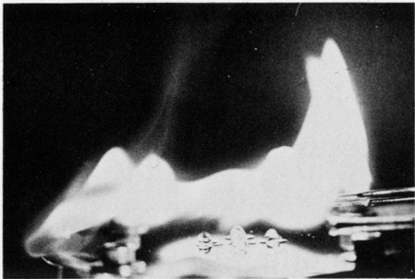
FIGURE 6. Ignition of a five-droplet array of n -heptane droplets (0.013 ml volume, L = 6 mm) on a stainless-steel surface at 250\text{ }^{\circ}\text{C} ( t = 0 s).
