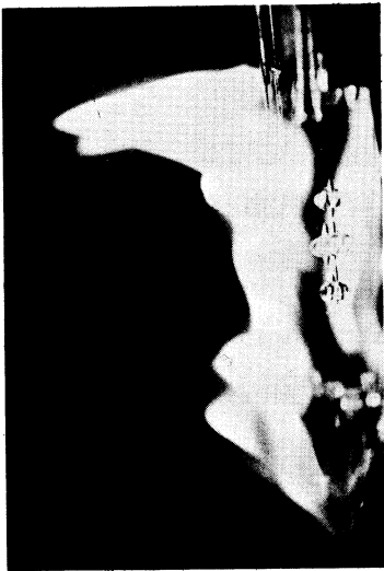
FIGURE 6. Ignition of a five-droplet array of n -heptane droplets (0.013 ml volume, L = 6 mm) on a stainless-steel surface at 250 °C ( t = 0 s).
