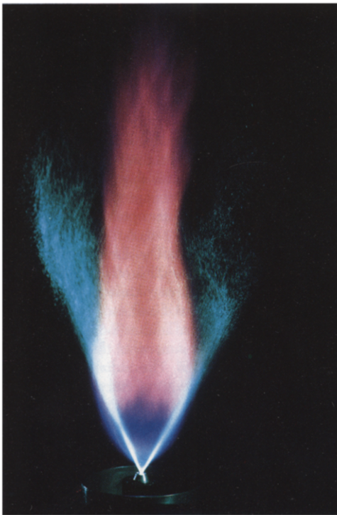
FIG. 2. Methanol flame illuminated by a vertical laser sheet beam.
