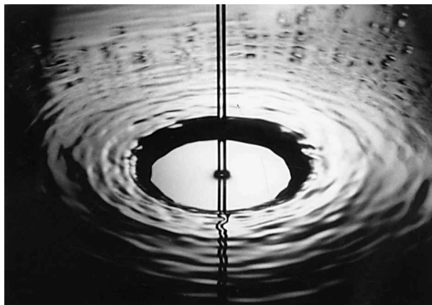
Figure 5. Photograph of a laminar water jet striking the target surface ( D_j = 2.54 mm; Q = 9.57 ml s ^{-1} ; h_\infty = 4 mm) at G = 1 . The water jet is the rod-like structure. The CHJ is the dark outer ring bounding the upstream thin film.
