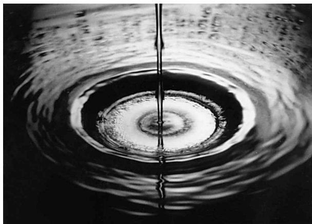
Figure 6. Photograph of the water jet in figure 5 taken 200 ms after the period of low gravity begins. The transition zone upstream of the CHJ has considerably thinned indicating reduced curvature of the free surface. A 'hump' or large wave is visible immediately downstream.
