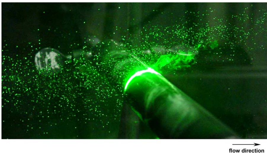
Fig. 16. View of the injected water spray over the heated cylinder.
