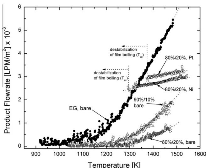
Fig. 7. Variation of product gas flow rate with average surface temperature for the mixtures examined on a bare tube, and Pt and Ni coated tubes. EG data are from Fig. 6. Dotted lines are included to show trends. Limits for collapse of film boiling are indicated for 80%EG/20% water mixtures with Pt and Ni catalyst coatings.
