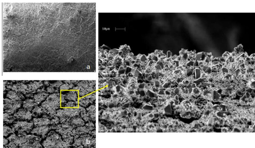
**Fig. 10.** SEM images of Ni catalyst surface before (a,b) and after (c) film boiling of an 80%EG/20% water mixture at 300X and 600X, respectively. (c) is an enlarged image of the Ni catalyst surface at 1800X.
