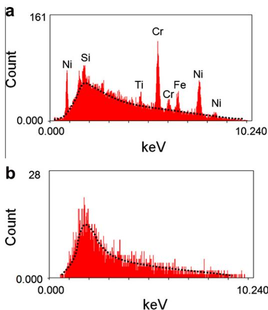
**Fig. 11.** X-ray diffraction scans of a bare Inconel tube (a) and a bare tube after film boiling in ethylene glycol (b). The tube after film boiling was coated with a black material (Fig. 10) that (b) indicates is non-metallic. The dotted line shows the baseline.
