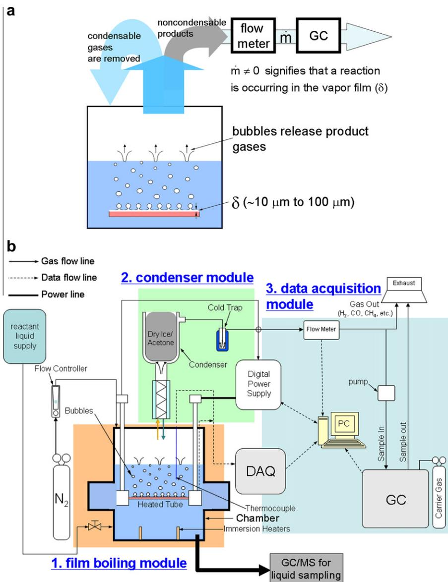
Fig. 3. (a) Schematic of gas flow paths in the experiment; (b) details of apparatus.
