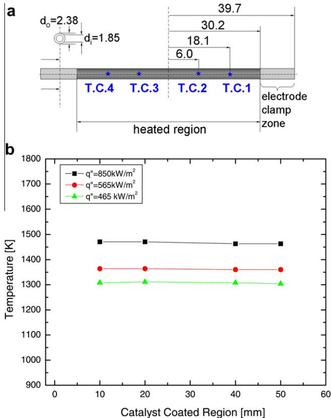
**Fig. 4.** (a) Schematic of tube assembly for film boiling showing locations of the thermocouples. The dimensions are in millimeters. Lightly shaded area of tube is in contact with electrode clamps and not exposed to reactant liquid. (b) Representative variation of surface temperature with distance along the tube for the locations in “a” at the three heat fluxes listed in the inset.
