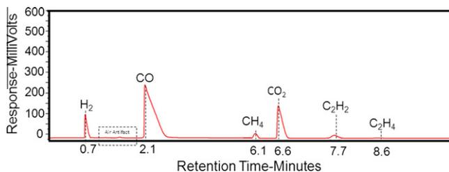
**Fig. 8.** GC trace for an 80%EG/20%water mixture for film boiling at an average tube surface temperature of 1373K with the following products and mole percents: H<sub>2</sub> (68.7%), CO (22.9%), CH<sub>4</sub> (1.1%), CO<sub>2</sub> (6.8%), C<sub>2</sub>H<sub>2</sub> (0.3%), and C<sub>2</sub>H<sub>4</sub> (0.1%).
