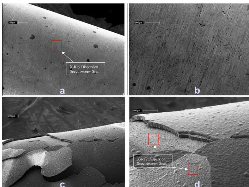
**Fig. 9.** SEM images of a bare tube (a) at 100X and (b) at 300X, for a tube before film boiling of a 90%EG/10%water mixture. SEM images after film boiling (c) at 100X and (d) at 300X. The boxes show where X-Ray dispersion spectroscopy scans were taken for Fig. 11.
