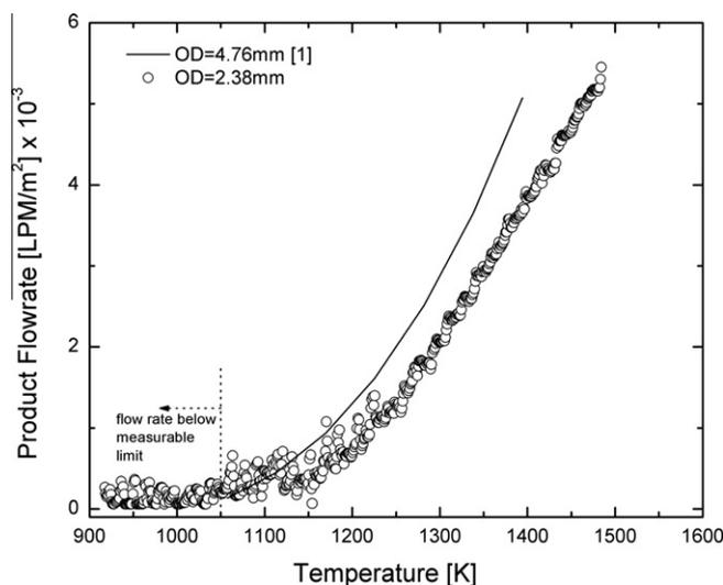
**Fig. 6.** Variation of measured product gas flow rates with average surface temperature for ethylene glycol. Line is average of data from [1] for a larger tube (4.76 mm O.D.). Lower film boiling limits are indicated for the 80%EG/20% water mixtures for the catalyst surfaces.
