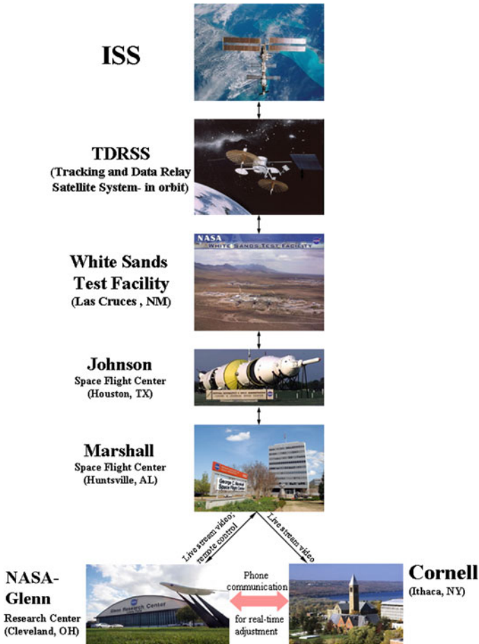
Fig. 7 Communication network for controlling operations on the MDCA. Hardware controls originate from NASA Glenn
