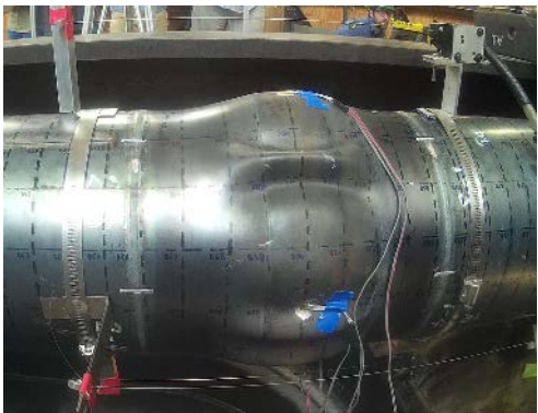
(f) 3.5 in. (89 mm) axial displacement
