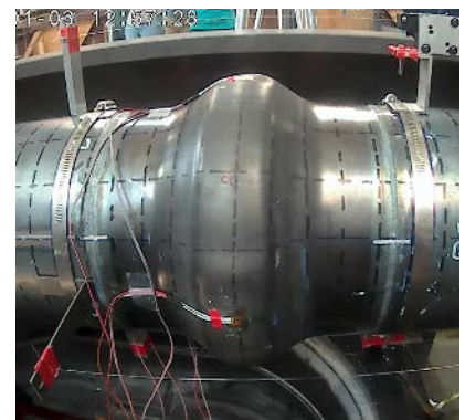
(i) +1.66 in. (+42 mm) Axial Displacement
