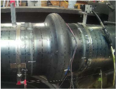
(b) 1 in. (25 mm) axial displacement
