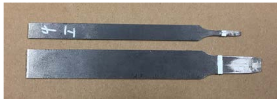
Figure 2.2. Size comparison of wall cut coupon specimens
