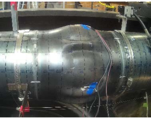
(e) 3 in. (76 mm) axial displacement
