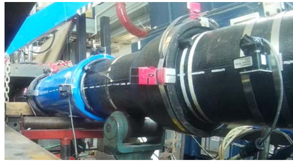
b) Joint Fully Extended and Locking Segments Rotated Inward
