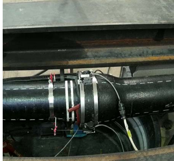
b) Joint Fully Extended and Locking Segments Rotated Inward
