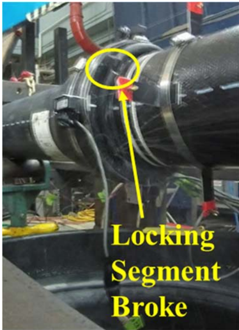
c) Left-Hand (Black) Locking Segment Broke
