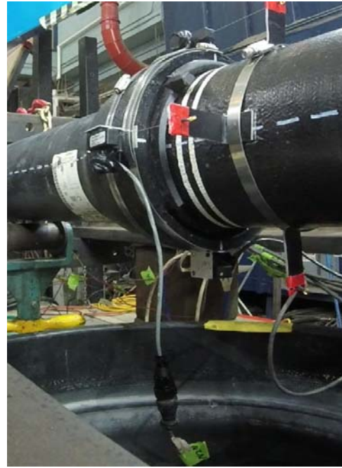
b) Joint Fully Extended and Locking Segments Rotated Inward
