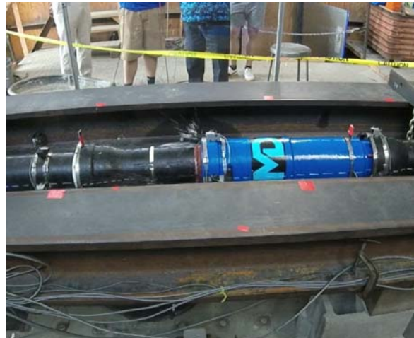
d) Pipe Leaked
