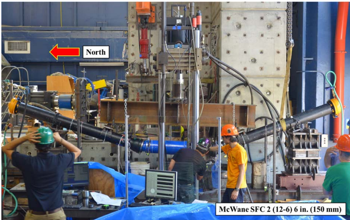
Figure 3.28. Photo of McWane SFC Bending Specimen 2 (12-6) after Testing
