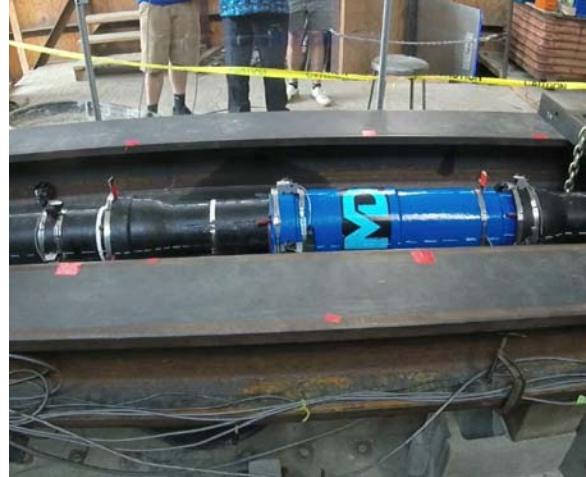
b) Joint Fully Extended and Locking Segments Rotated Inward
