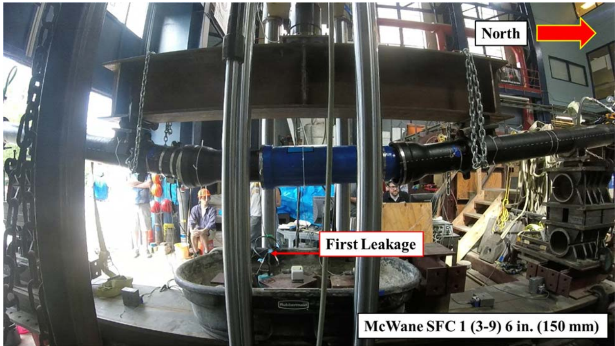
Figure 3.17. First Leakage of McWane SFC Bending Test Specimen 1 (3-9)
