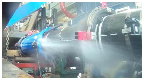
d) Pipe Leaked
