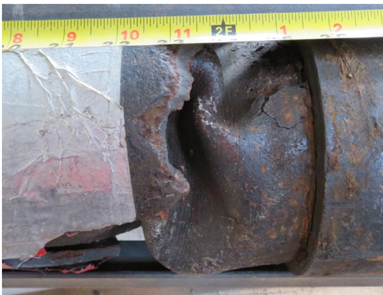
Figure 6.10. DC2 Deformed and Buckled Lining
