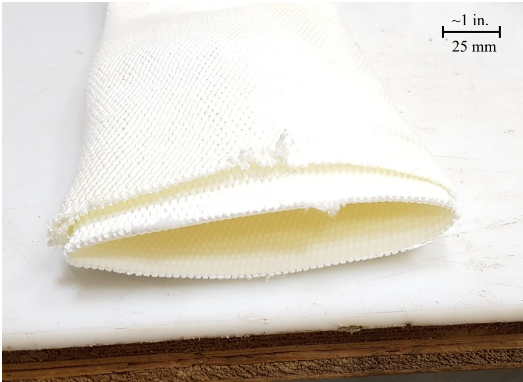
Figure 1.3. Aqua-Pipe™ Generation 1 (AP1) Woven Fabric Lining before Curing
