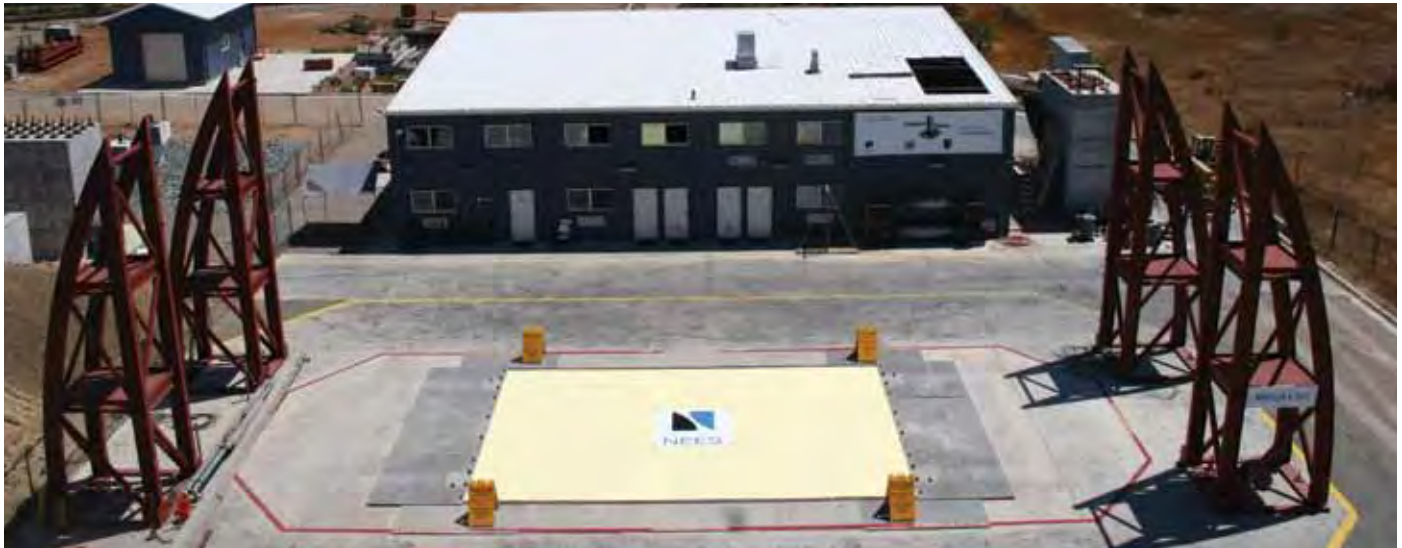
The Large High Performance Outdoor Shake Table is one of the largest shake tables in the world.
