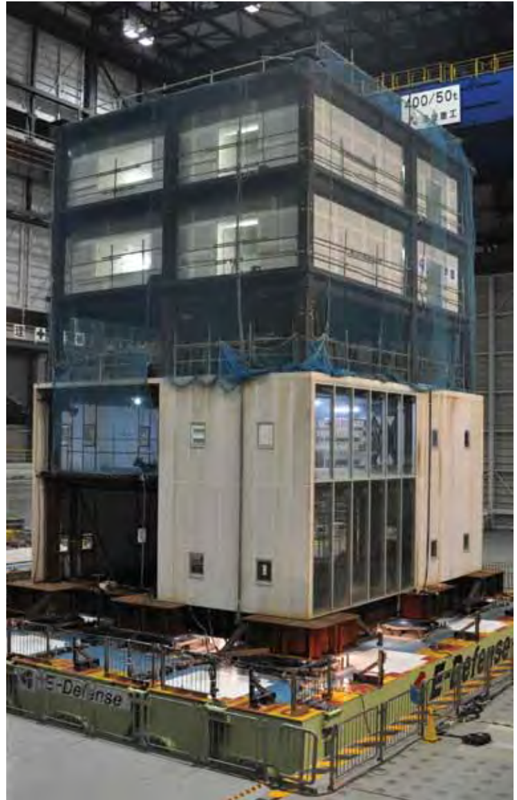
At E-Defense, shake table tests were performed on a 5-story full scale steel moment frame building isolated with triple pendulum bearings. The isolation system consisted of 9 bearings, one beneath each column of the building.
