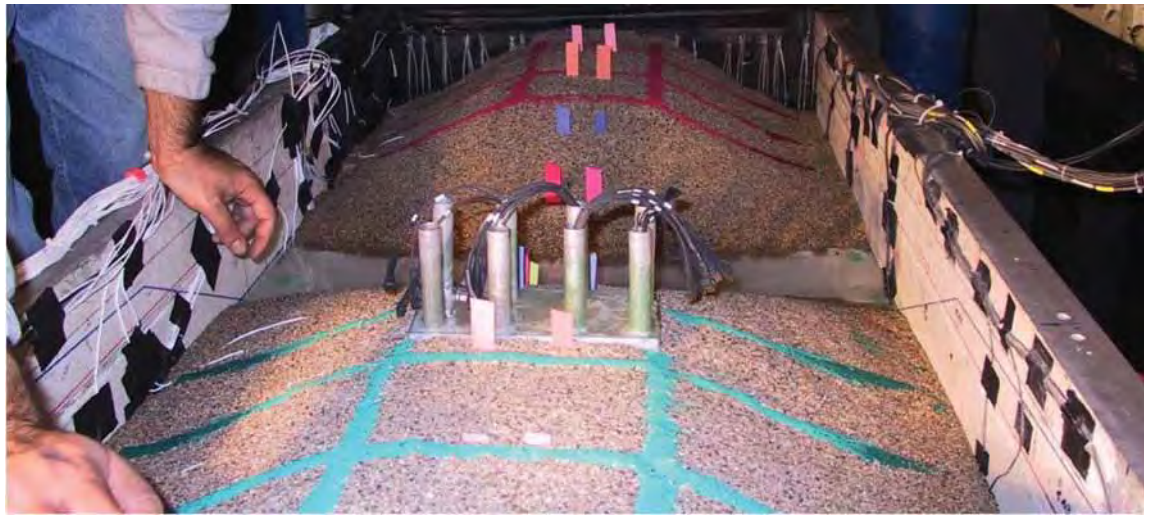
Centrifuge model of two opposing approach embankments; the embankment in the foreground includes a pile group, whereas the embankment for the background does not.
