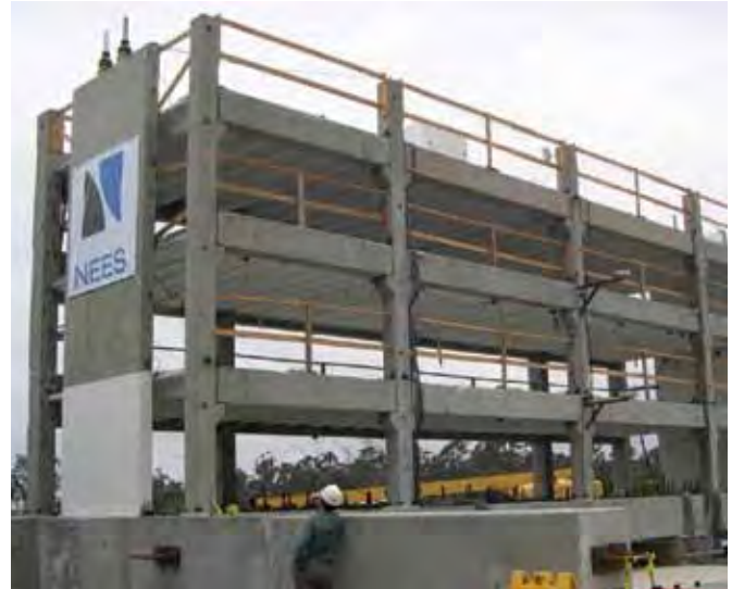
Half-scale shake table test at the NEES at UC San Diego facility.
