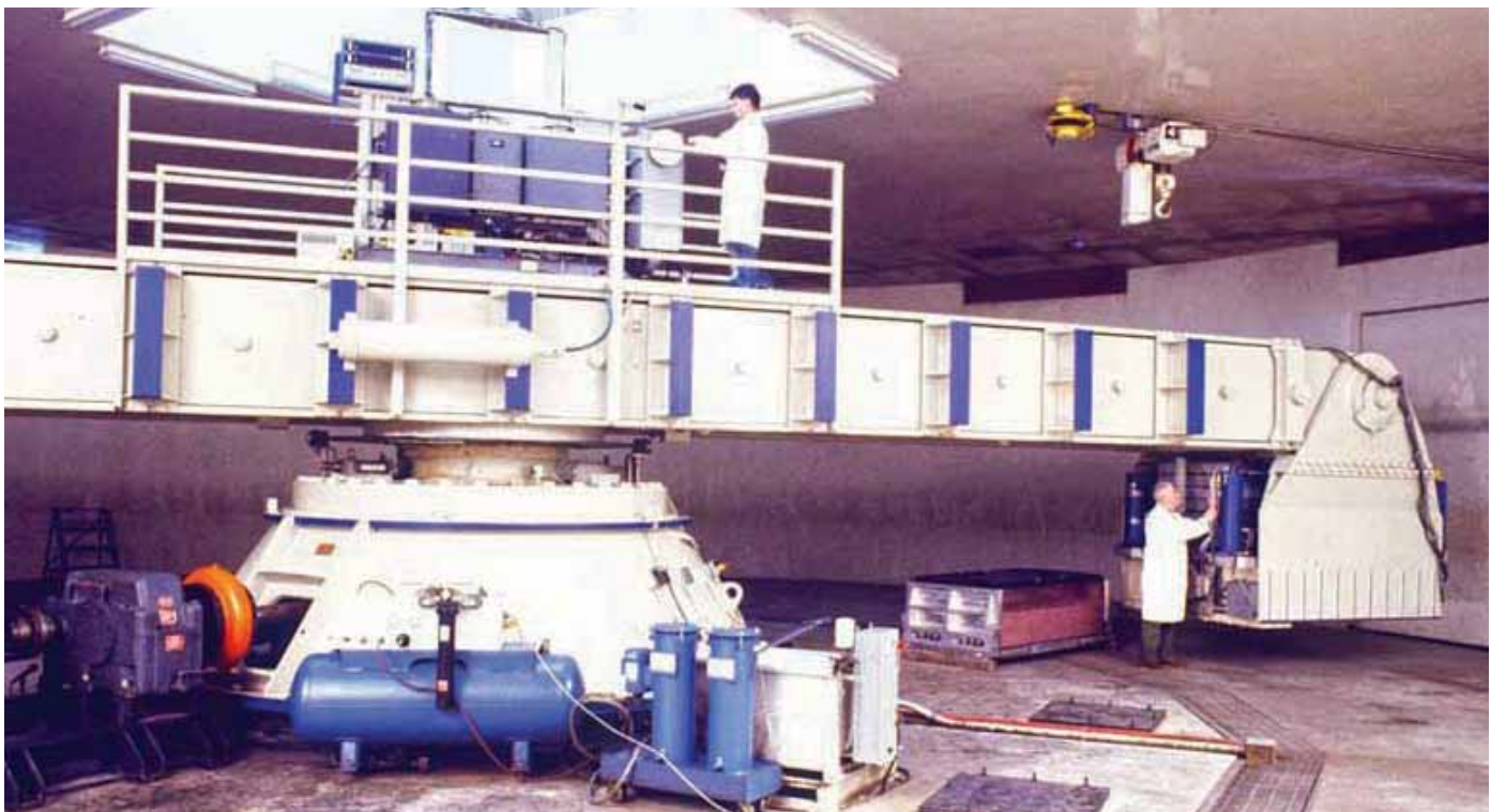
The UC Davis centrifuge has the largest radius and platform area of any geotechnical centrifuge in the United States and is among the largest in the world.
