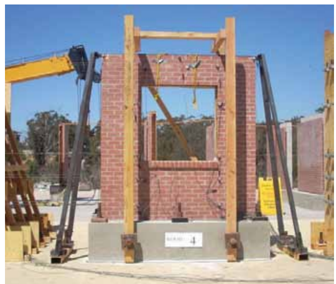
In-plane testing of an 8 x 8 foot wall to determine the effects of corrugated ties and joint reinforcement.
