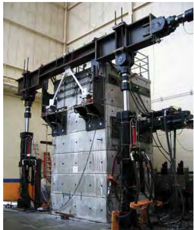
Reconfigurable reaction wall being used to test a suspended zipper frame.
