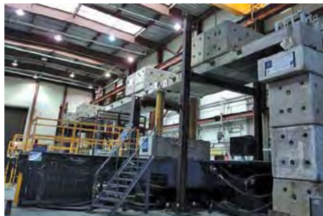
View of the bridge after installation of superimposed mass.
