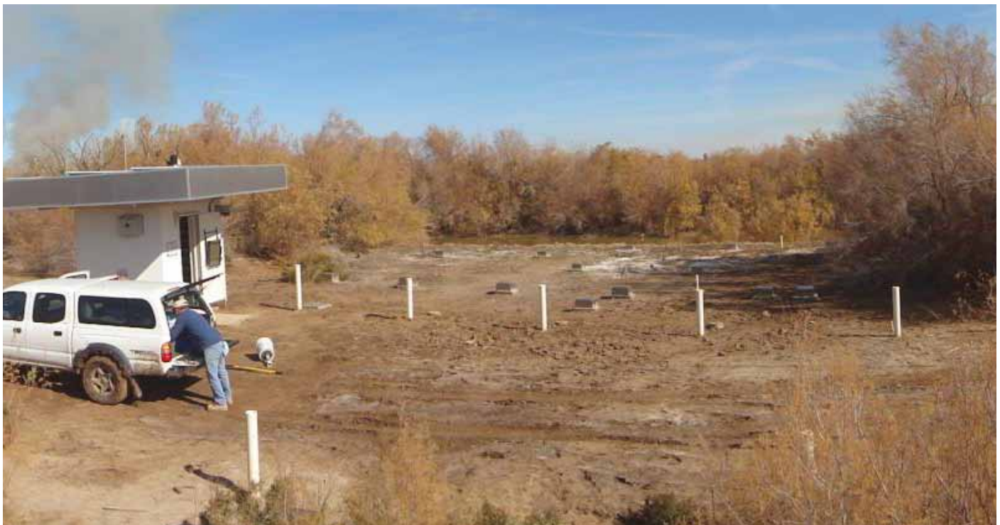
The Wildlife Liquefaction Array records numerous earthquakes daily.
