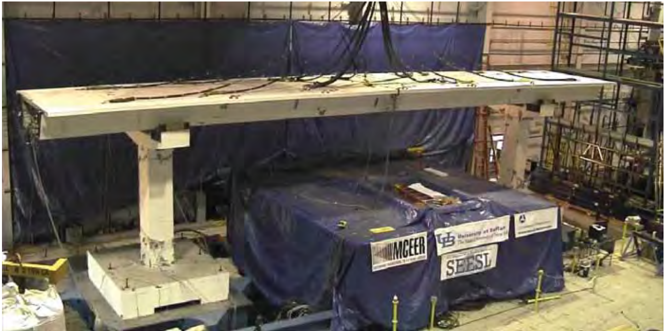
A large scale bridge model was designed according to the Accelerated Bridge Construction techniques.
