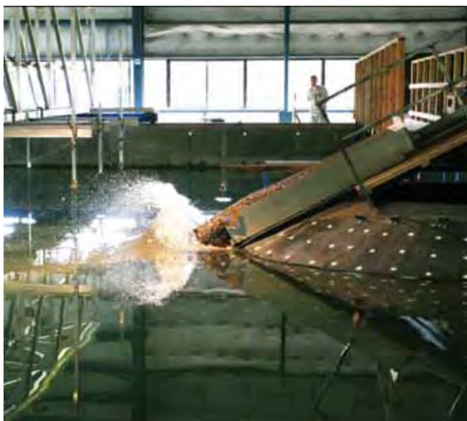
Landslide impact creates the first wave crest.
