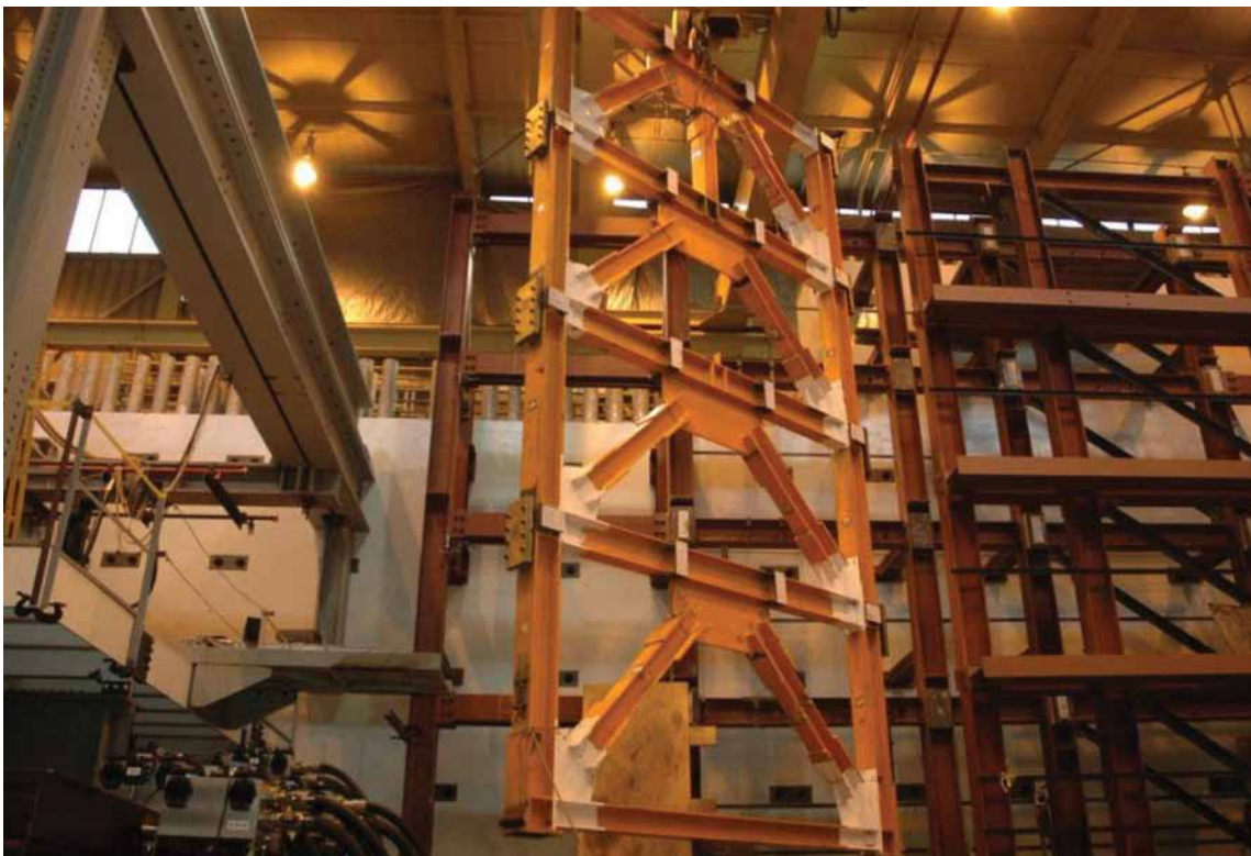
A self-centering concentric braced frame is maneuvered into place for testing.
