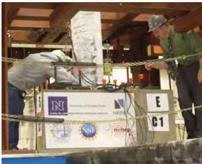
Project PI David Sanders (right) inspects a column specimen at the NEES at University of Nevada, Reno facility.
