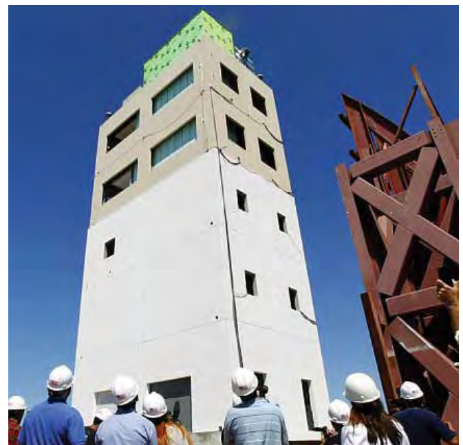
Engineers and members of the media watch a specially constructed five-story building during an earthquake test in San Diego.
