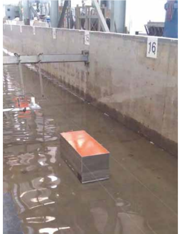
A 1:5 scale model shipping container in the Oregon State Wave Flume, waiting for the tsunami.
