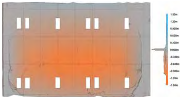
Deformation analysis for the Gamou Wastewater treatment plant after impact by the the 2011 Tohoku Tsunami. The histogram on the right shows the distribution of various levels of change across the wall.
