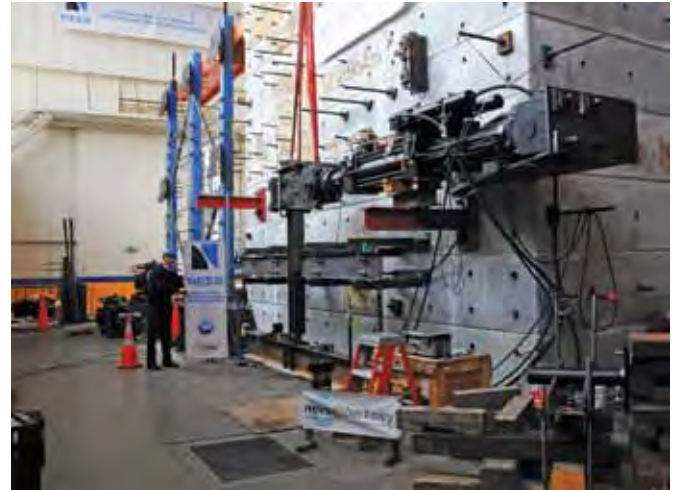
A hydraulic actuator installed on a station on NEES at Berkeley's reconfigurable reaction wall. Site Manager Shakhzod Takhirov is pictured.
