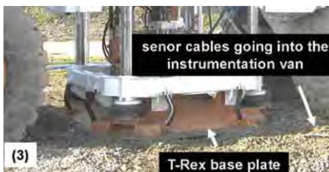
Preparing for T-Rex shaking: (1) Burying sensor cables in native soil; (2) placing gravel pad; (3) load with T-Rex overnight, and (4) T-Rex shaking and recording.
