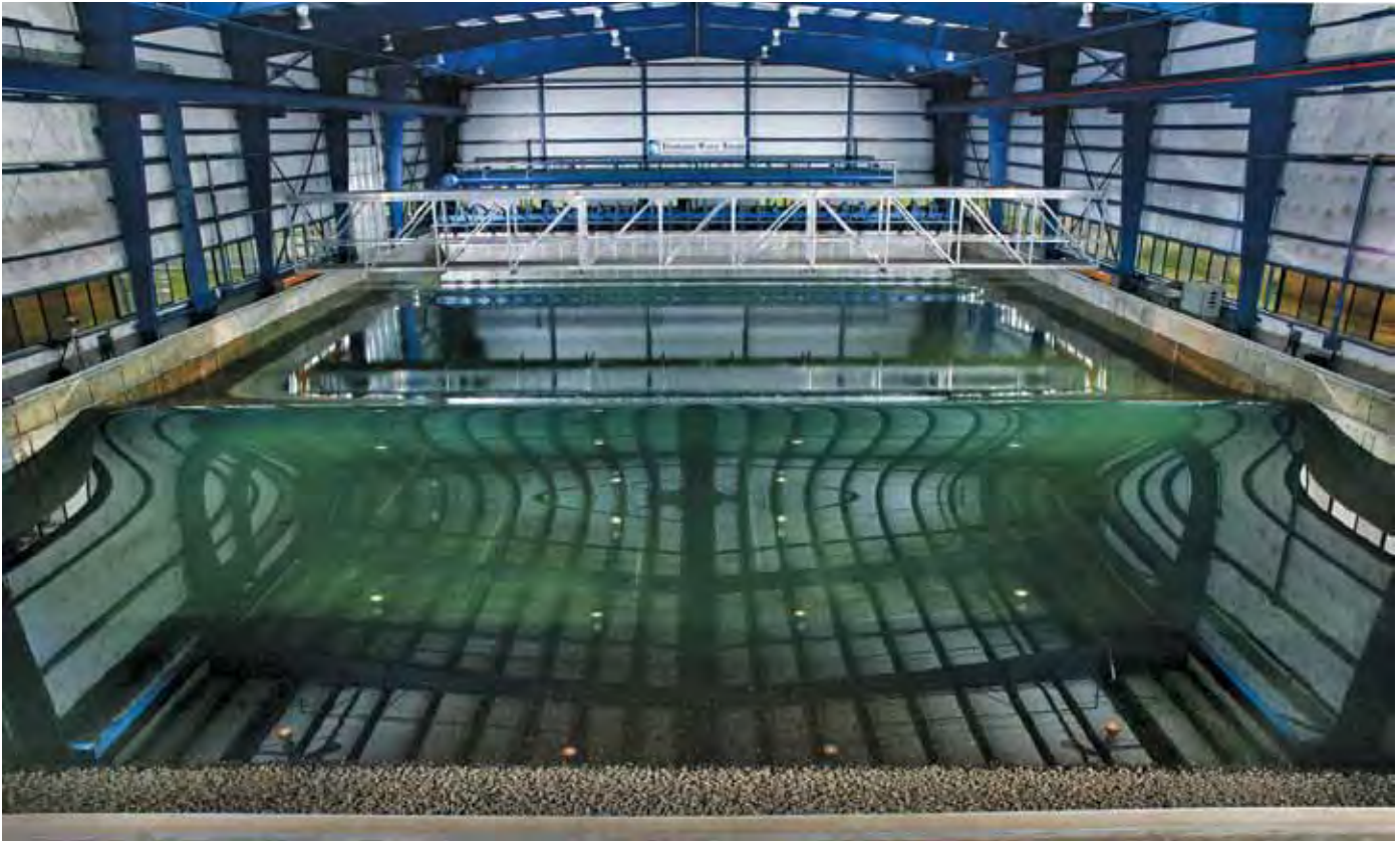
The Tsunami Wave Generator at NEES at Oregon State University.
