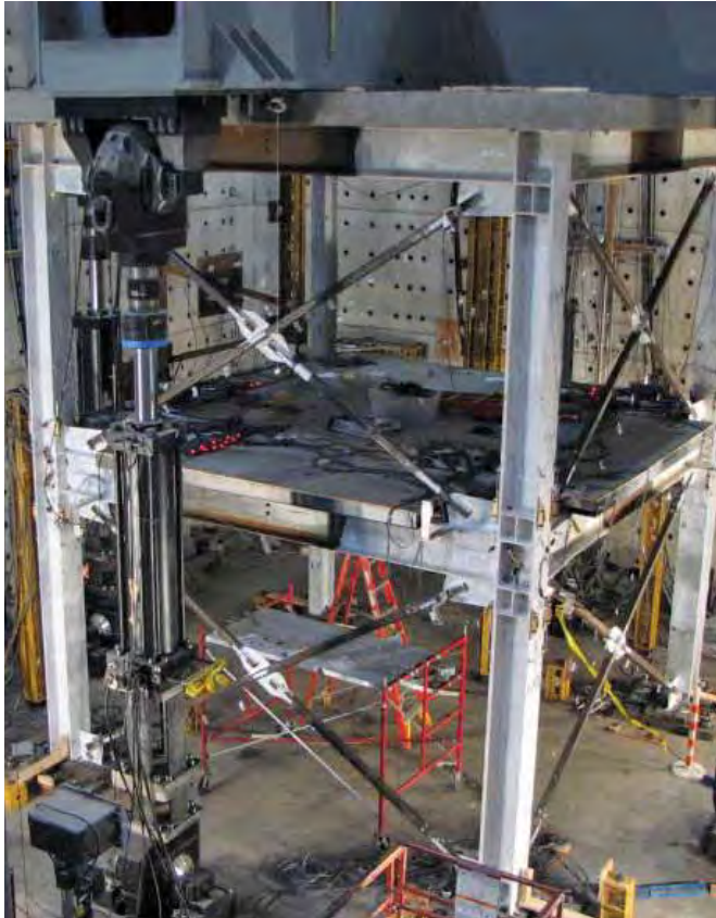
Full-scale 3-D Braced Frame test specimen ready for testing in the MAST laboratory.
