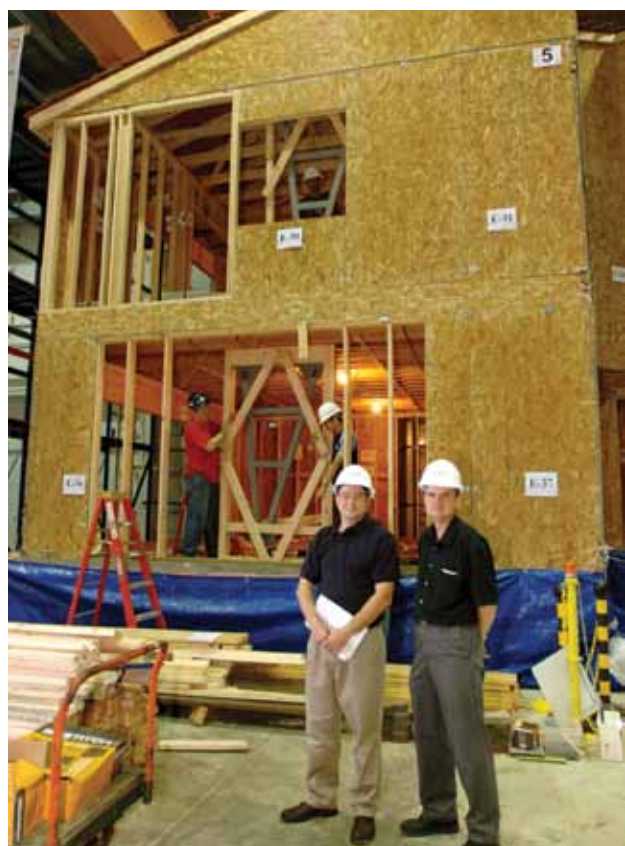
Andre Filiatrault of UB (right) and Michael Symans of Rensselaer Polytechnic Institute tested seismic dampers in a full-scale wood-frame house in UB's Structural Engineering and Earthquake Simulation Laboratory.
