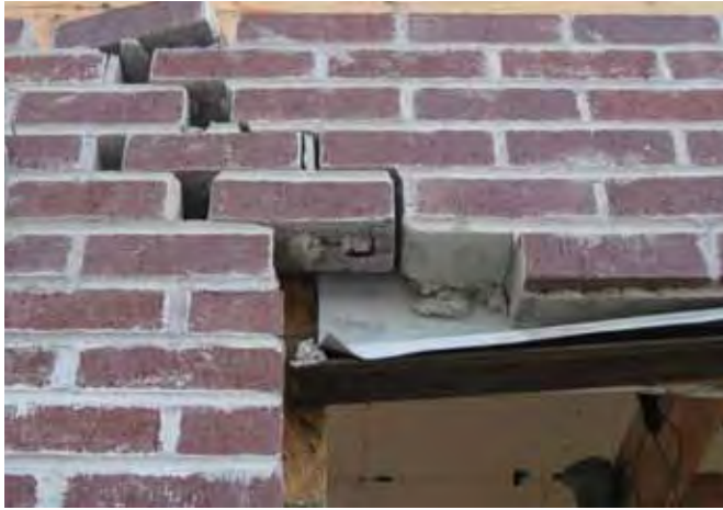
Damage caused by the shake test.
