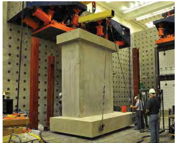
C-Shaped Wall #3. This test was the final specimen in the project, which included seven prior tests at NEES at Illinois.
