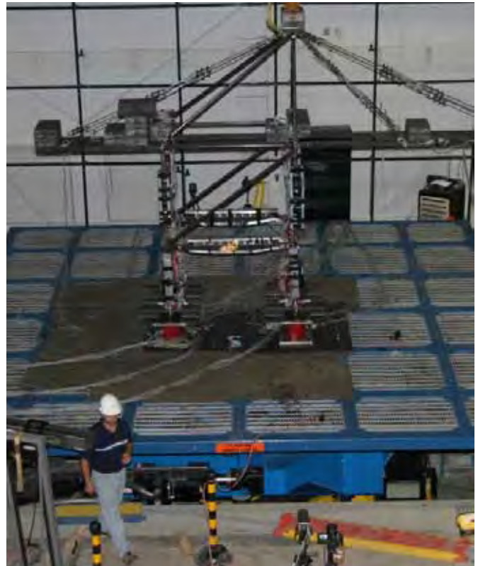
1/20th scale crane on the shake table at the NEES at Buffalo facility.
