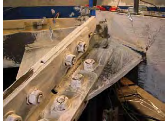
The cracked gusset-to-column weld after testing.
