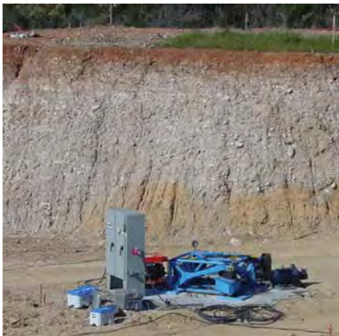
Testing with the MK-15 eccentric mass shaker at Elliot Field.
