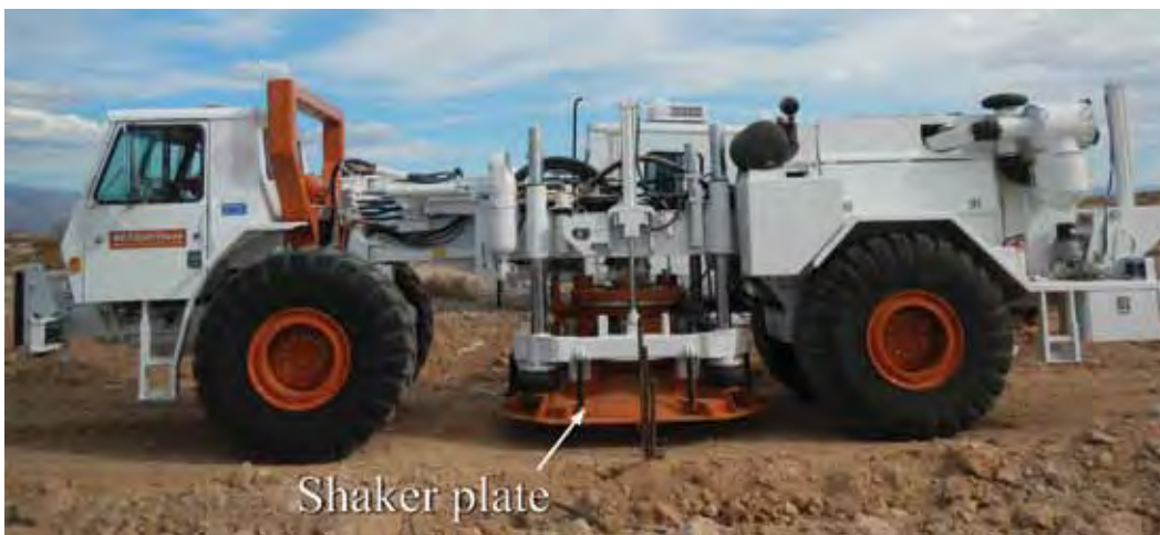
A mobile field shaker simulating earthquake shaking in an Arizona landfill.
