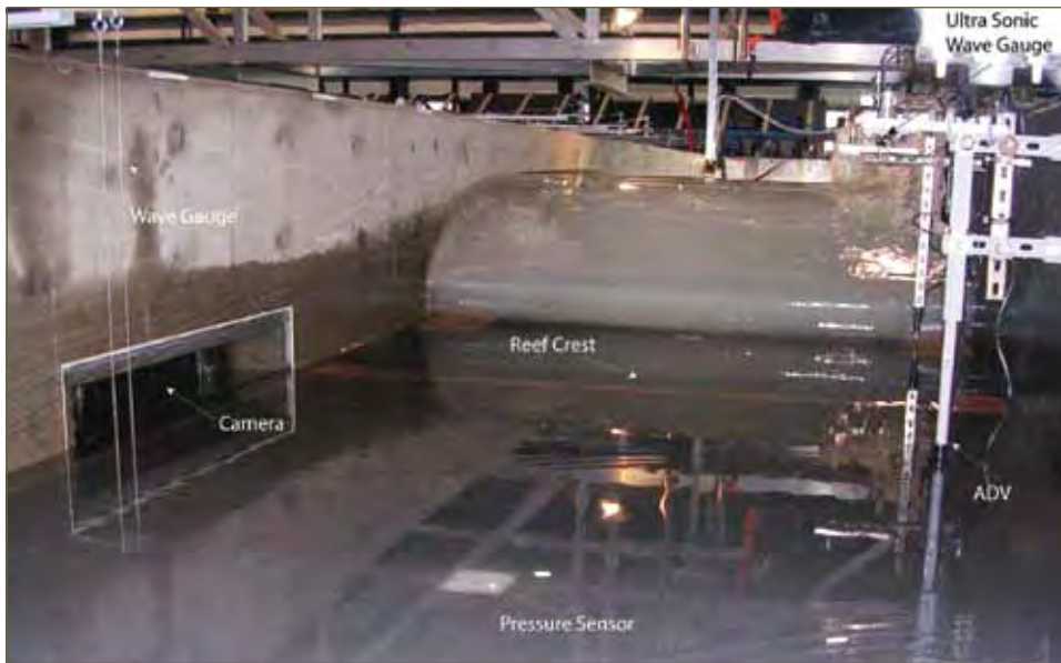
Wave propagating down the wave flume at the NEES at Oregon State facility.
