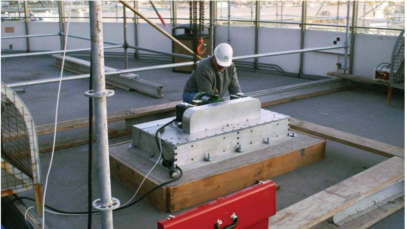
NEES at UCLA used the "Mighty Mouse" shaker to validate the Los Angeles International Airport Theme building retrofit.
