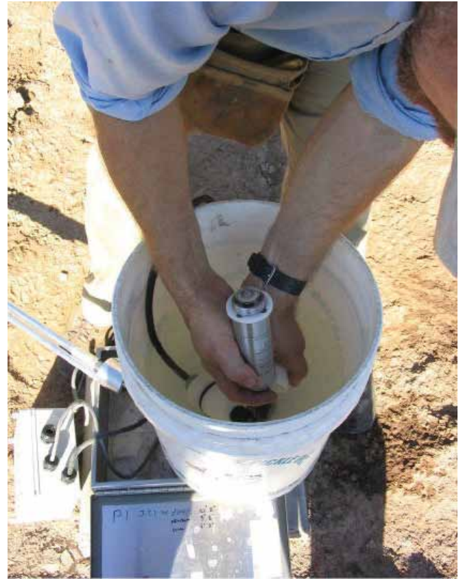
Pressure transducer being saturated in a bucket of water in preparation for installation of the assembly in the casting below the bucket.
