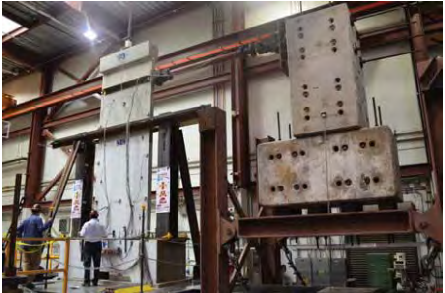
Shake table test setup used at NEES at UNR for SRWs and PreWEC systems.
