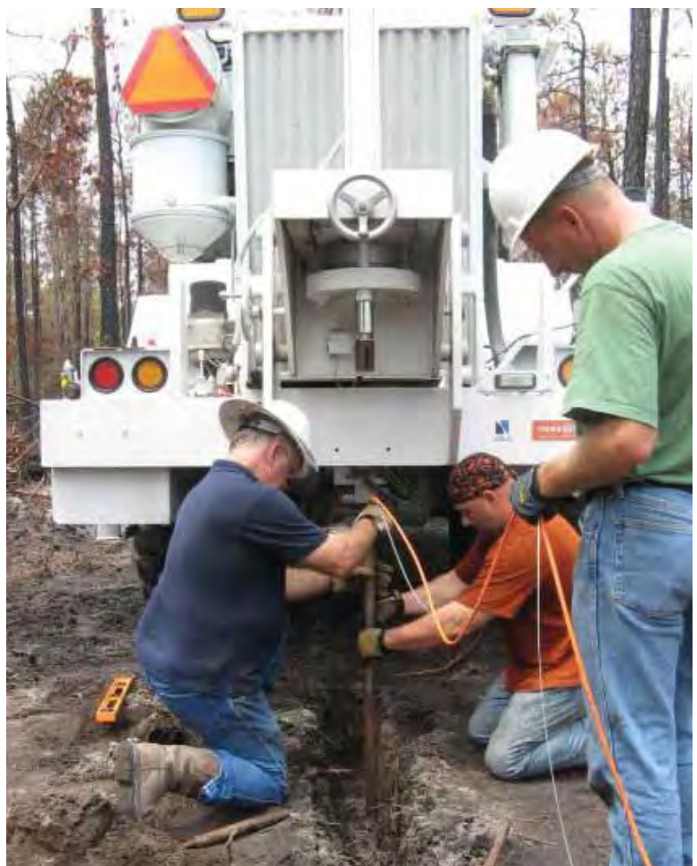
Field instrumentation measures excess pore pressure.
