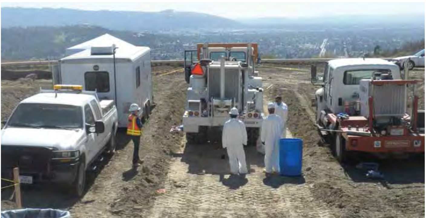
The T-Rex being used to evaluate the dynamic properties of municipal solid waste.
