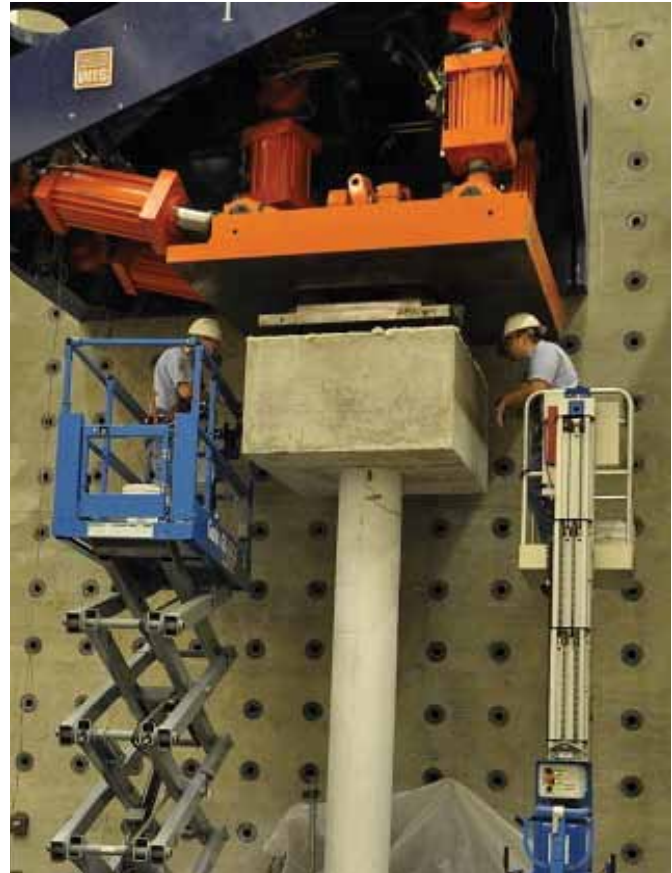
One of three Loading and Boundary Condition Boxes mounted on the strongwall for the CABER connect.
