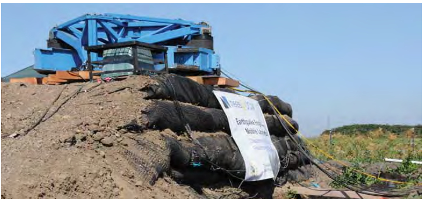
The NEES at UCLA eccentric mass shaker sits atop a model levee.
