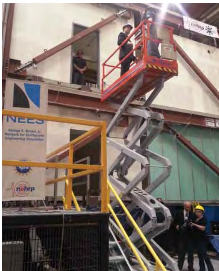
The capstone test at the NEES at University of Nevada, Reno facility. A full-scale, 2 story building filled with nonstructural components was subjected to earthquake motions.
