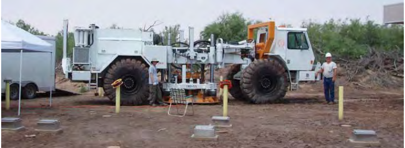
T-Rex in position to apply horizontal dynamic loads to an embedded array of sensors at the NEES Wildlife Liquefaction Array.
