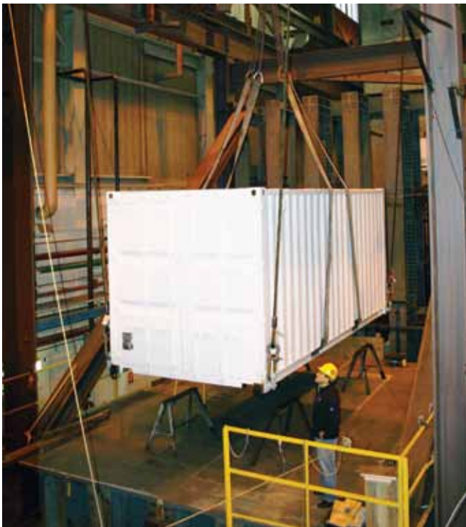
Shipping container in pendulum test setup at Lehigh University being inspected by Prof. Clay Naito.
