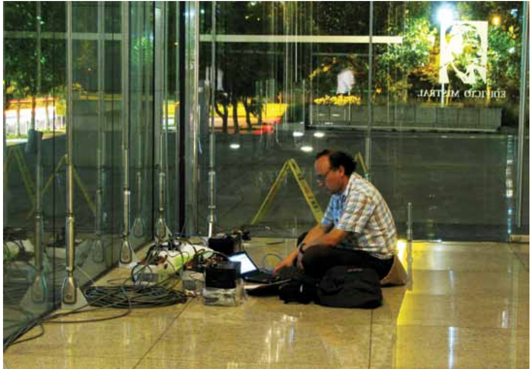
NEES at UCLA engineer Alberto Salamanca operating the temporary monitoring system in the Mistral Building.
