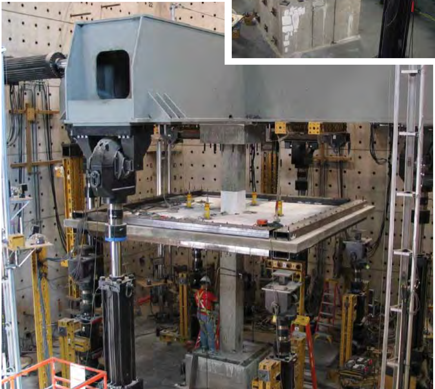
Minnesota's Multi-Axial Subassembly Testing (MAST) Laboratory is comprised of a strong floor and a 94,000 pound steel cross head which allows earthquake engineers to test a variety of specimens, such as beam-column joints, multi-story frames, and walls.
