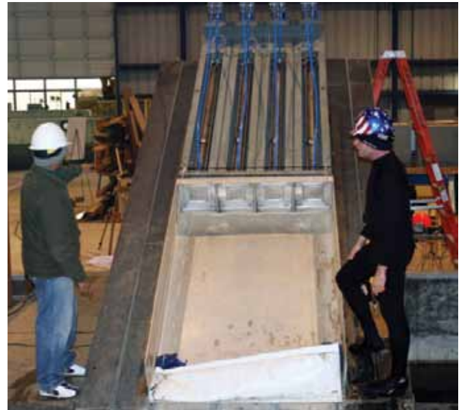
The team's novel pneumatic landslide simulator allows for controlled acceleration and shape of the granular landslide material. It consists of a sled which is driven by four pneumatic pistons.
