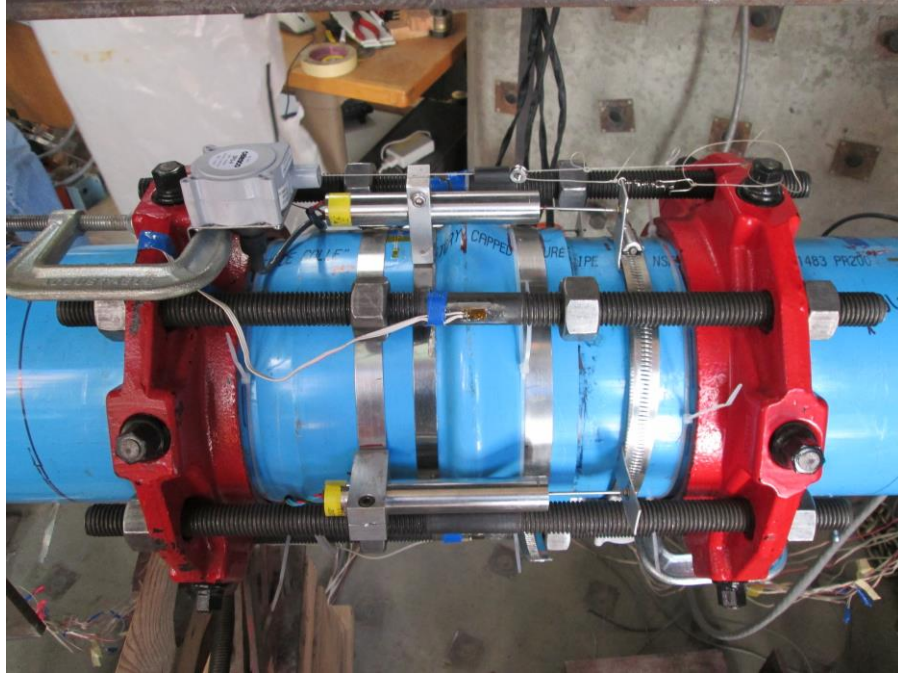
Photo B.5. Test RT3 Joint Instrumentation
