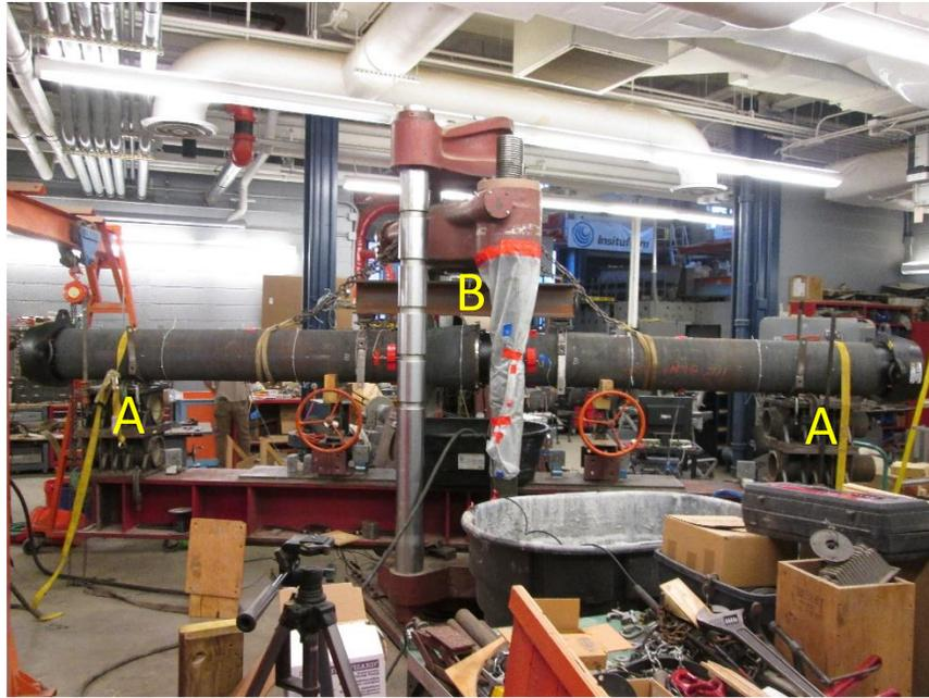
Figure 2.8. Four-Point Bending Test Apparatus
