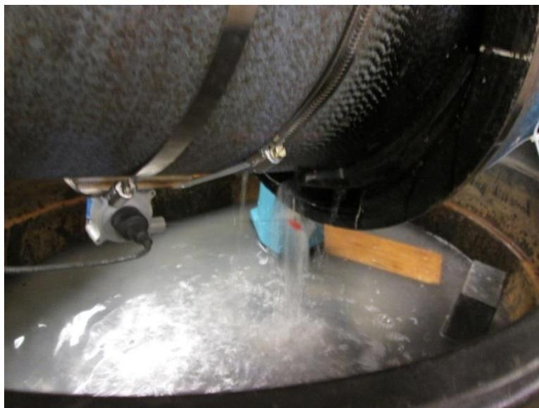
Figure 2.7. Final Leakage of Test A
