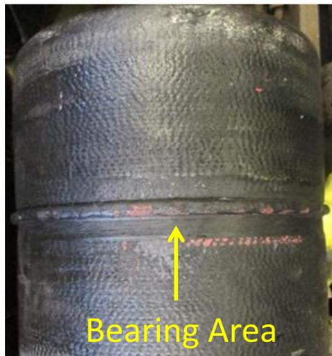
Figure 3.9. Restraining Clips Bearing Area on the Spigot of Test 1
