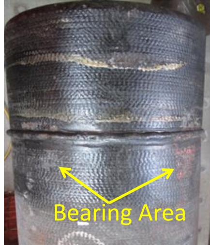
Figure 3.19. Restraining Clips Bearing Area on the Spigot of Test 2
