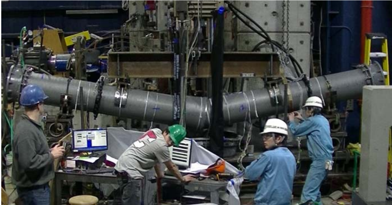
Figure 2.32. Photo of 16-in. (400-mm) ERDIP Bending Specimen T4 after Testing
