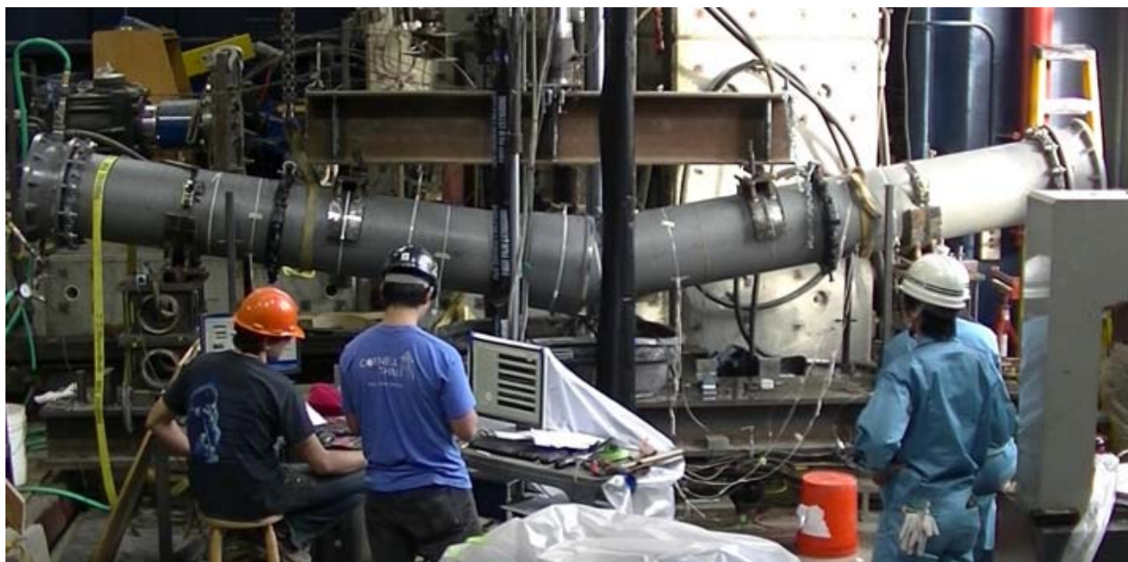
Figure 2.24. Photo of 16-in. (400-mm) ERDIP Bending Specimen T3 after Testing
