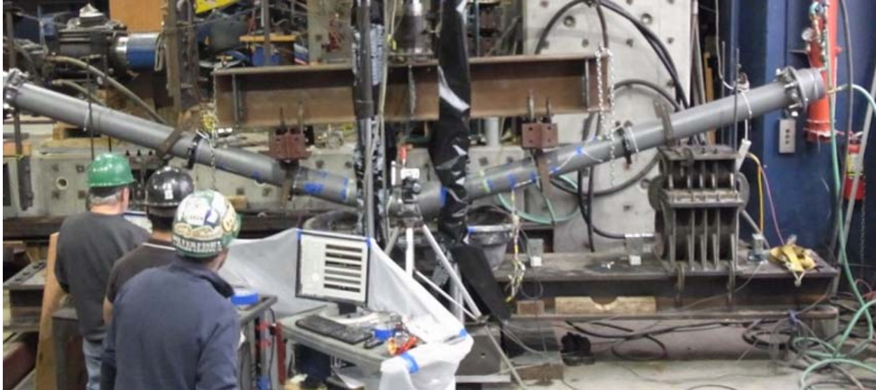
Figure 2.8. Photo of 6-in. (150-mm) ERDIP Bending Specimen T1 after Testing
