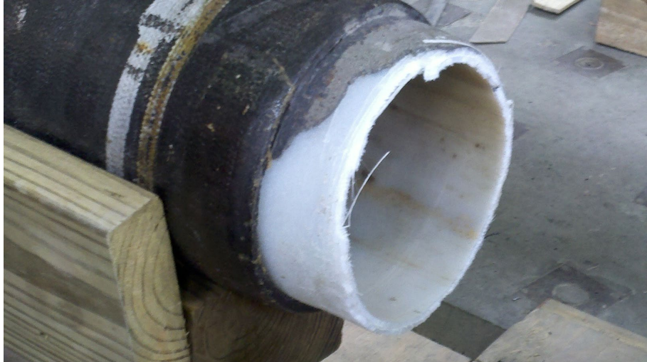
Photo 6. Specimen No. 8, Bonded Liner, Joint Pull Test
