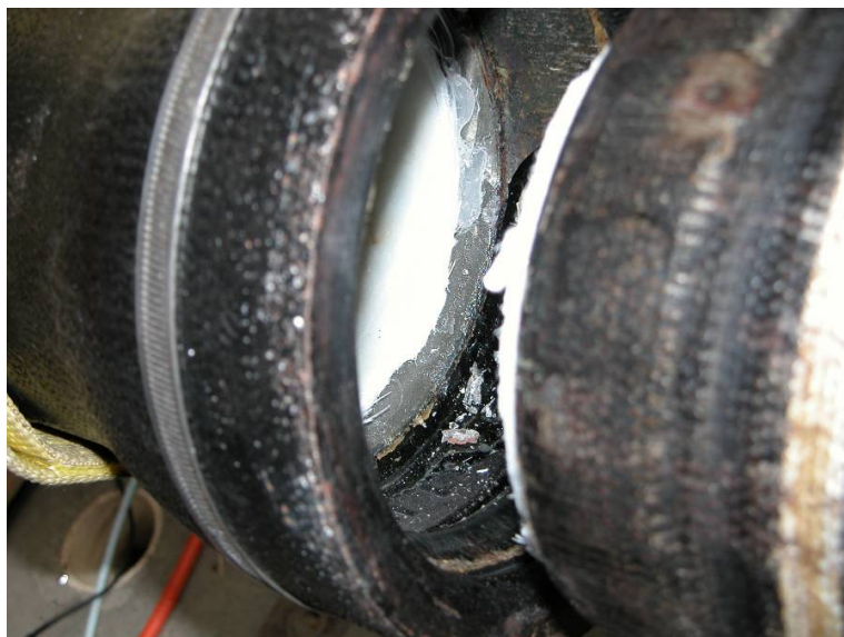
Photo 3. Specimen No. 4, Unbonded Liner, Joint Pull Test
