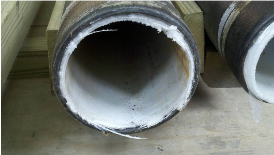
Photo 8. Specimen No. 11, Bonded Liner, Joint Pull Test, Spigot End
