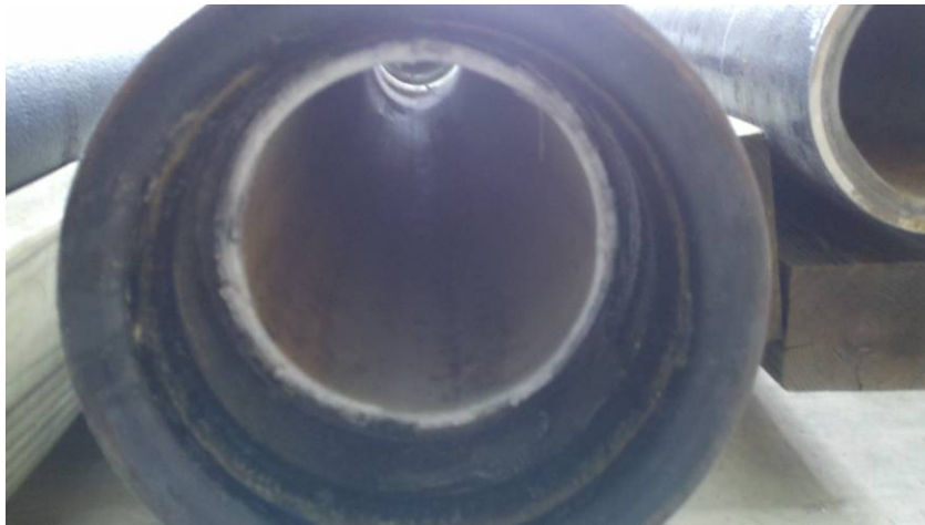
Photo 7. Specimen No. 11, Bonded Liner, Joint Pull Test, Bell End
