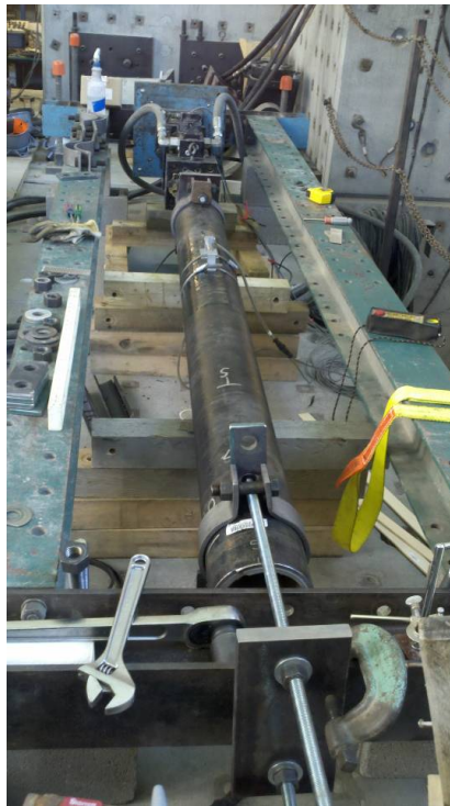
Photo 1. Experimental Setup for Lined Pipe Pullout Testing
