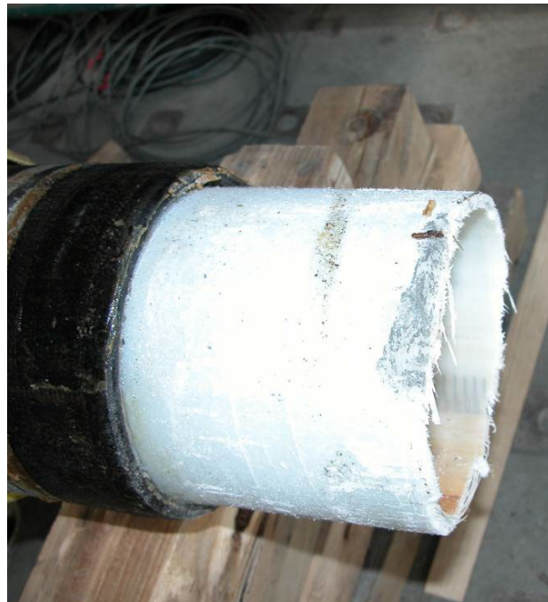
Photo 5. Specimen No. 9, Bonded Liner, Joint Pull Test
