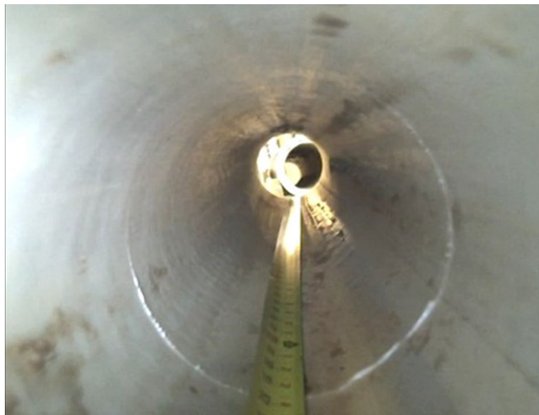
Photo 3. Image of the Specimen 2 Liner after First Rotation Testing Showing a Crack at the Center
