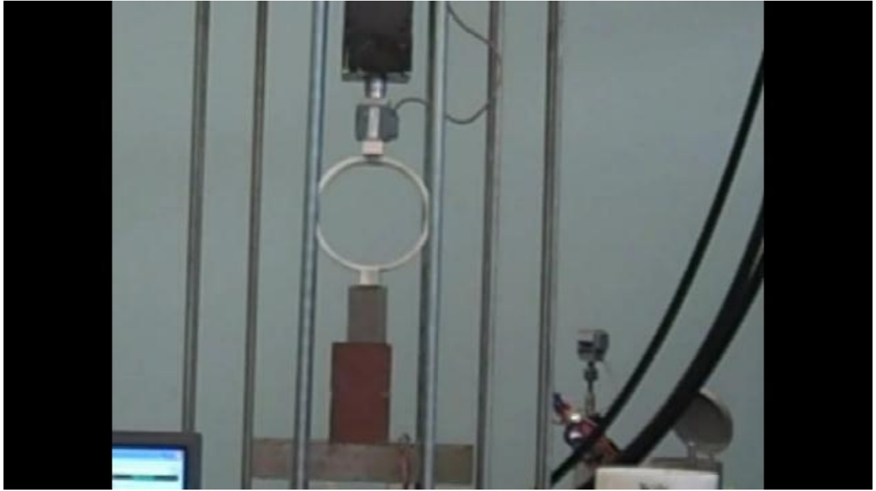
Photo 5. Ring 1S Prior to Test to Failure
