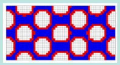
A typical distribution of material with spherical obstructions present in the fluid can be modelled using  $\epsilon$
