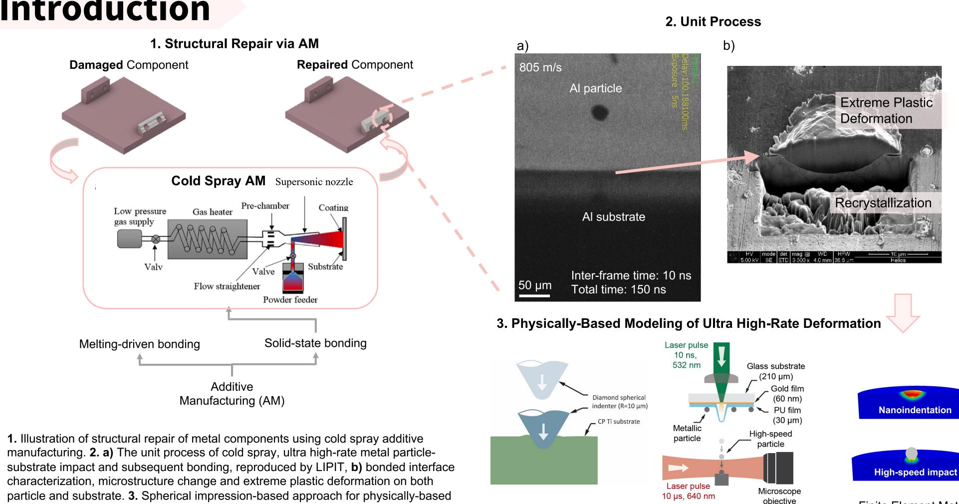
manufacturing. 2. a) The unit process of cold spray, ultra high-rate metal particlesubstrate impact and subsequent bonding, reproduced by LIPIT, **b**) bonded interface characterization, microstructure change and extreme plastic deformation on both particle and substrate. **3.** Spherical impression-based approach for physically-based constitutive modeling of materials in ultra high-rate deformation.
