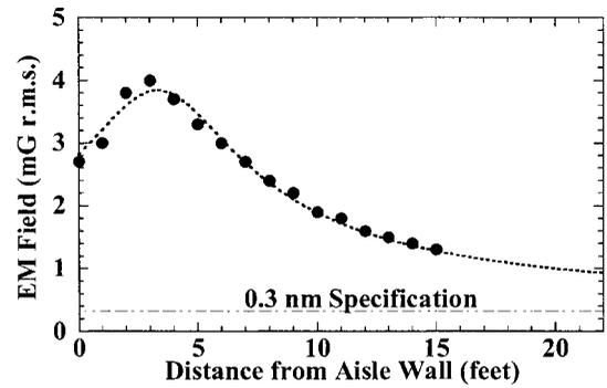
**Fig. 3** The measured magnetic field from a power bus located 3 feet below the floor (closed circle). The fit (dotted line) to Ampere's law is for 1.5 mA current flowing at  $x = 3.3$  feet and 2.9 feet below the floor. The bus was rerouted.
