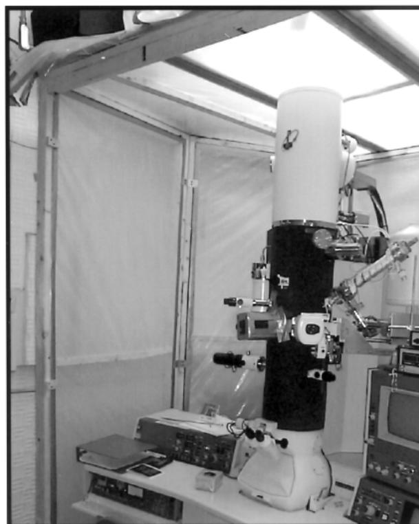
**Fig. 7** A ‘gazebo’ shelters the microscope from cross-drafts produced by the air conditioning, and neoprene rubber around the column and stage damps out pressure and temperature fluctuations.
