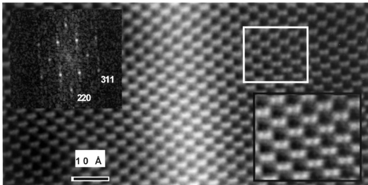
**Fig. 10** An ADF-STEM image of a Sb  $\delta$ -layer in [110] oriented Si, showing an information limit better than 0.163 nm and minimal drift during the 40 s acquisition. The peak Sb concentration is 20 atoms or about 0.2 monolayers. (JEOL 2010F at 197 kV,  $C_s = 1$  mm,  $\theta_0 = 10$  mr, and low-pass filtered.)
