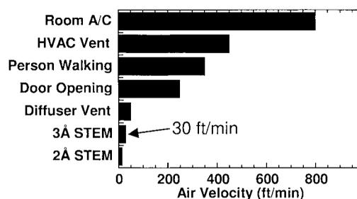
**Fig. 5** Maximum airflow across the microscope column that can be tolerated for sub 0.3 and 0.2 nm STEM compared with common causes of drafts.
