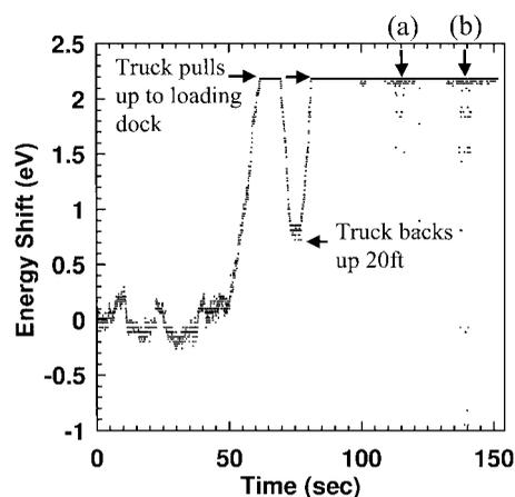
**Fig. 4** Deflection of the zero-loss peak on the post-column energy loss spectrometer as a truck pulls up to the loading dock outside the microscope room. The signal is clipped at 2 eV. The truck is first detected at about 50 feet away ( $t \sim 55$  s). It pulls up to the loading dock, and then backs up to come in straight. The spikes at (a) and (b) correlate well with the driver opening his door (a) and dropping the tailgate of the truck (b).
