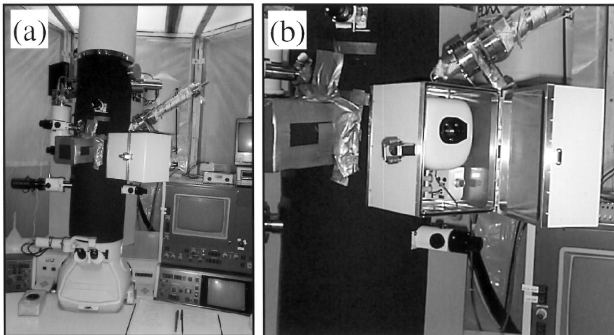
**Fig. 9** Adding an airtight airlock cover reduced the pressure sensitivity problem of Fig. 8. (a) The airlock cover is closed. (b) The airlock cover is open, showing the O-ring seal needed to isolate the specimen rod from rapid pressure changes in the room. Note that the stage drive to the left of the airlock is covered with neoprene for improved thermal stability.
