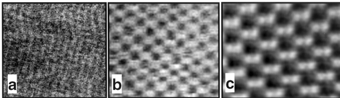
**Fig. 1** Annular dark-field STEM images of [110] oriented silicon, recorded (a) when the microscope was first installed, (b) after 6 months and (c) after 1 year. The improvement in image quality from (a) to (b) was from improvements in the instrument, and from (b) to (c) was due to improvements in the room environment.
