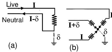
**Fig. 2** The origin of ground currents in (a) a single phase circuit and (b) a three-phase circuit. The net AC field generated by the conductors will be proportional to the current,  $\delta$ , lost to ground.
