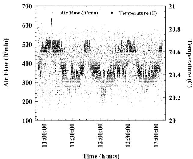
**Fig. 6** Airflow and air temperature recorded at the air return vent of the microscope room. The air is well mixed so this temperature reflects the temperature changes in the room. The airflow rate and size of the return allowed us to calculate the mass of air moving through the room, and, hence, its heat removal capacity.
