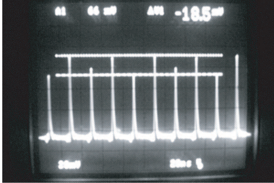
Figure 6.11: The pulse train recorded from the NPE rejection port showing the laser in stable, single-pulse mode-locked operation with a periodicity of 4T_R .
