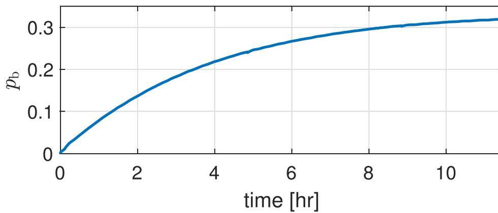
**Extended Data Fig. 1 | Spin-exchange optical pumping.** Typical measurement of the pumping process of helium-3 by optically pumped potassium vapor. Here the potassium density is  $n_a = 4.9 \cdot 10^{14} \text{ cm}^{-3}$ , and the helium depolarization time is  $T_{1,\text{act}}^b = 3.9 \text{ h}$ .
